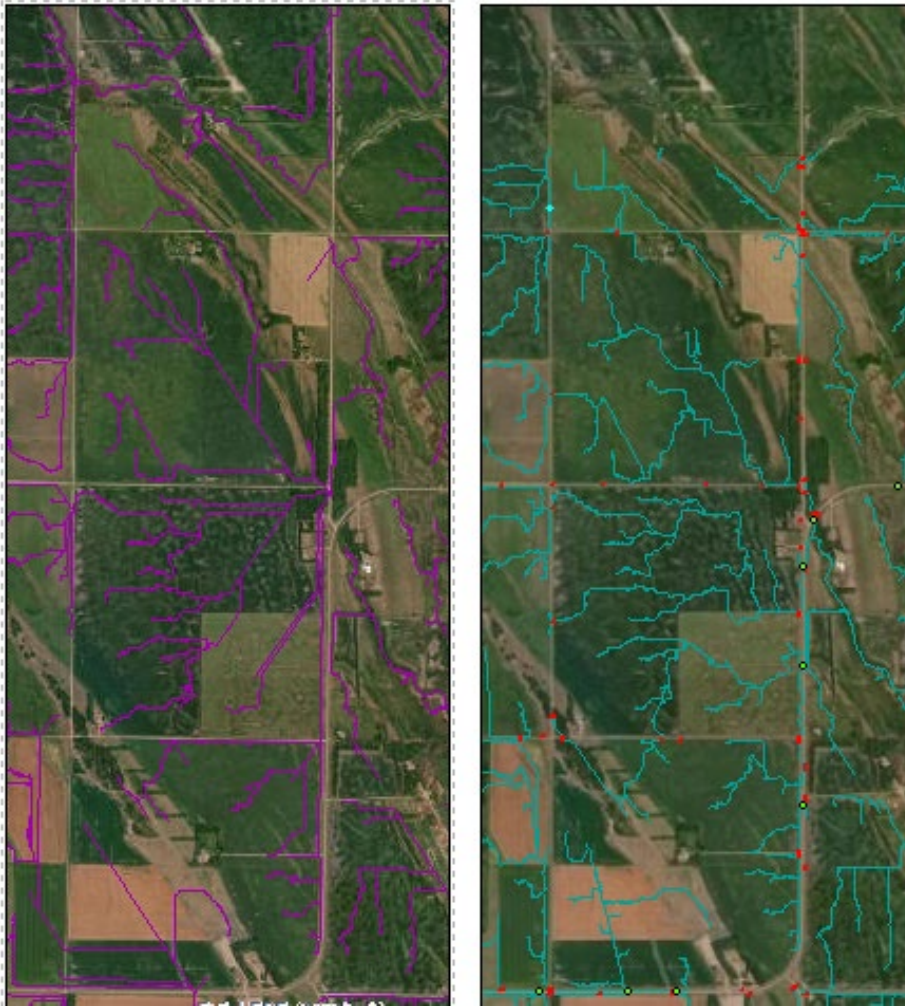
Figure 2. Left panel shows incorrect surface flow network that results if no culverts are hydroenforced. Right panel shows a correct surface flow network that results when culverts from the ND DOT culvert inventory (green dots) and other culverts identified by GIS tools (red lines) have been hydroenforced.
