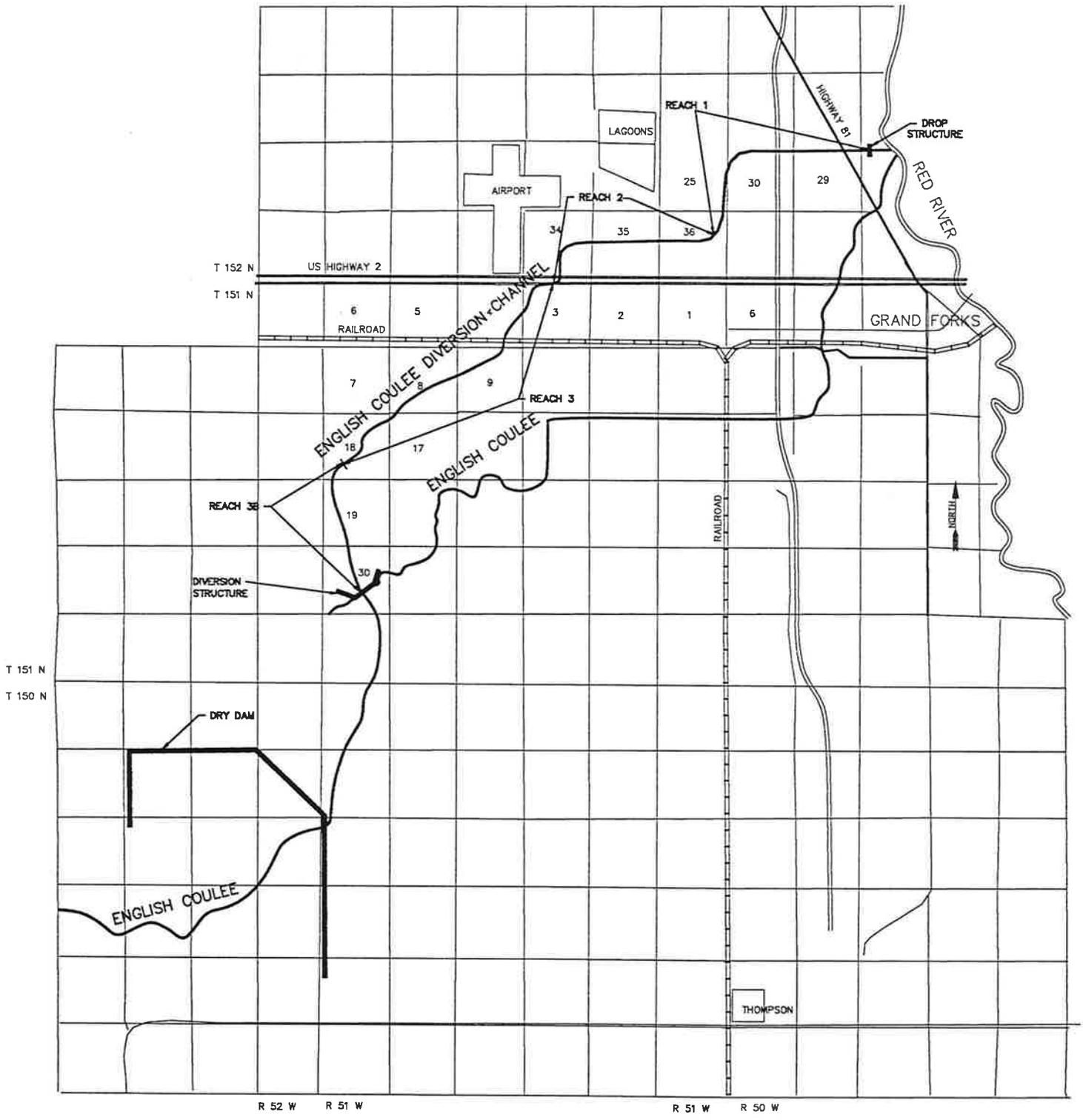
Figure 2 - Map Showing Channel Alignment and Reaches Used in HEC-2 Model
