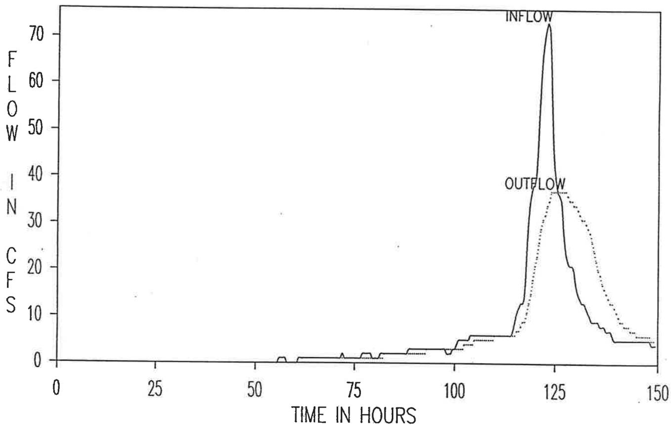
Figure 6 - Belfield Dam Hydrograph
