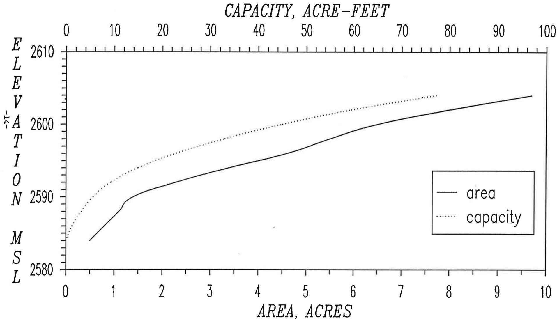
Figure 4 - Area-Capacity Curve
