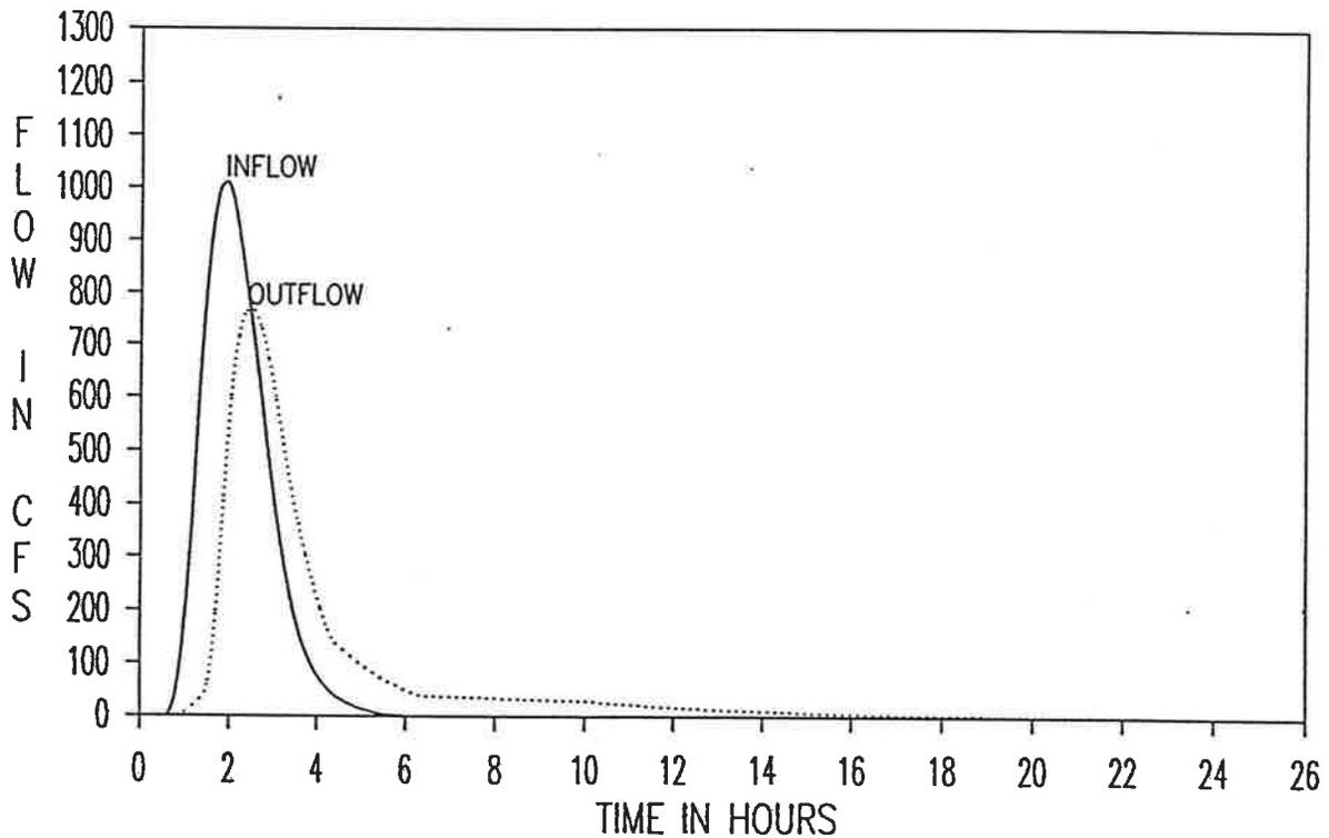
Figure 7 - Belfield Dam Hydrograph
