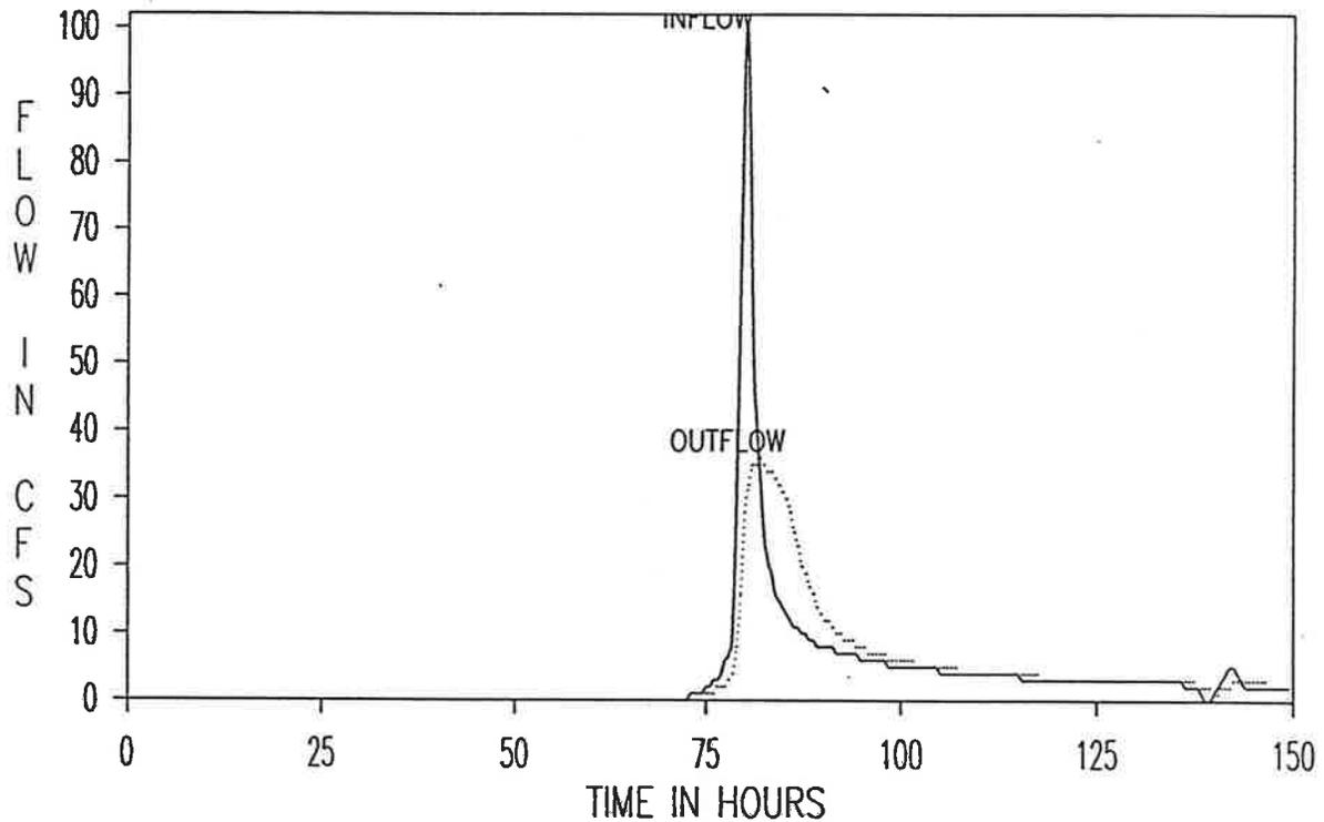
Figure 5 - Belfield Dam Hydrograph
