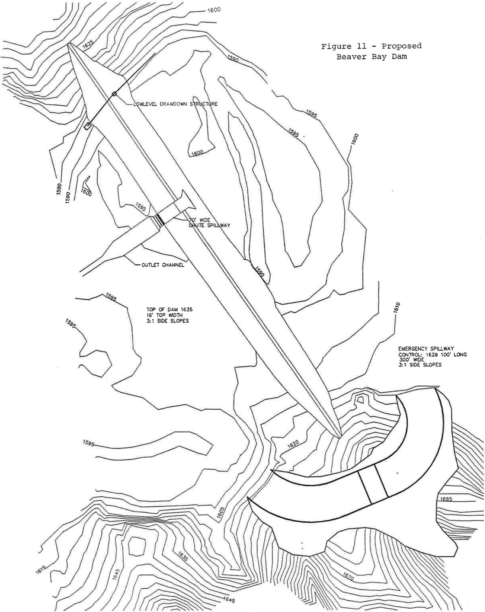
designed to counteract accelerated aging in reservoirs. The low-level drawdown structure removes nutrient-rich water from the bottom of a thermally stratified reservoir, leaving the better quality water behind, and thus increasing the usefulness and life span of the reservoir. Improved water quality conditions result in a positive benefit to the fishery and to all other recreational uses.
