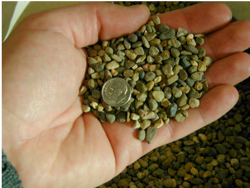
Figure 28. Photo of filter pack used in the production well construction.
