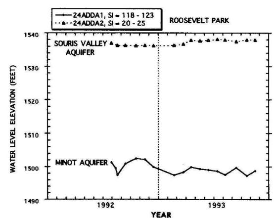
FIGURE 33. Hydrographs of water levels from piezometer nest 155-083-24ADD showing the vertical distribution of water levels in the Souris Valley and Minot aquifers.
