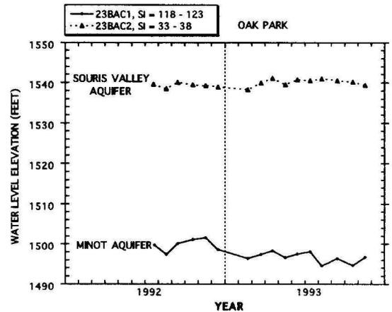
FIGURE 31. Hydrographs of water levels from piezometer nest 155-083-23BAC showing the vertical distribution of water levels in the Souris Valley and Minot aquifers.
