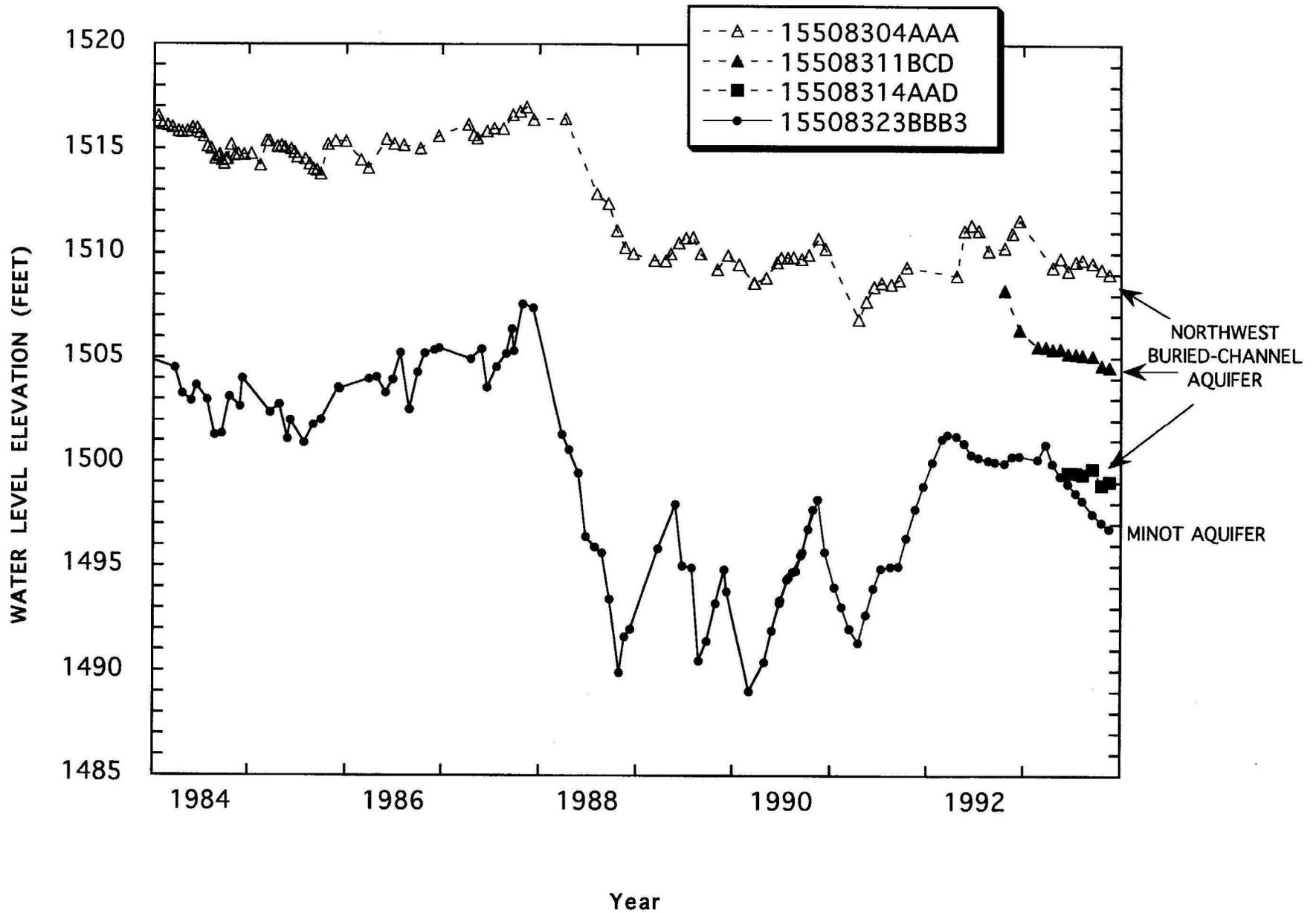
FIGURE 15. COMPARISON OF WATER LEVELS IN THE MINOT AQUIFER AND WATER LEVELS IN THE NORTHWEST BURIED-CHANNEL AQUIFER
