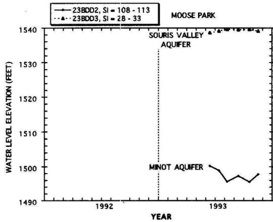
FIGURE 32. Hydrographs of water levels from piezometer nest 155-083-23BDD showing the vertical distribution of water levels in the Souris Valley and Minot aquifers.
