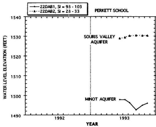
FIGURE 30. Hydrographs of water levels from piezometer nest 155-083-22DAB showing the vertical distribution of water levels in the Souris Valley and Minot aquifers.
