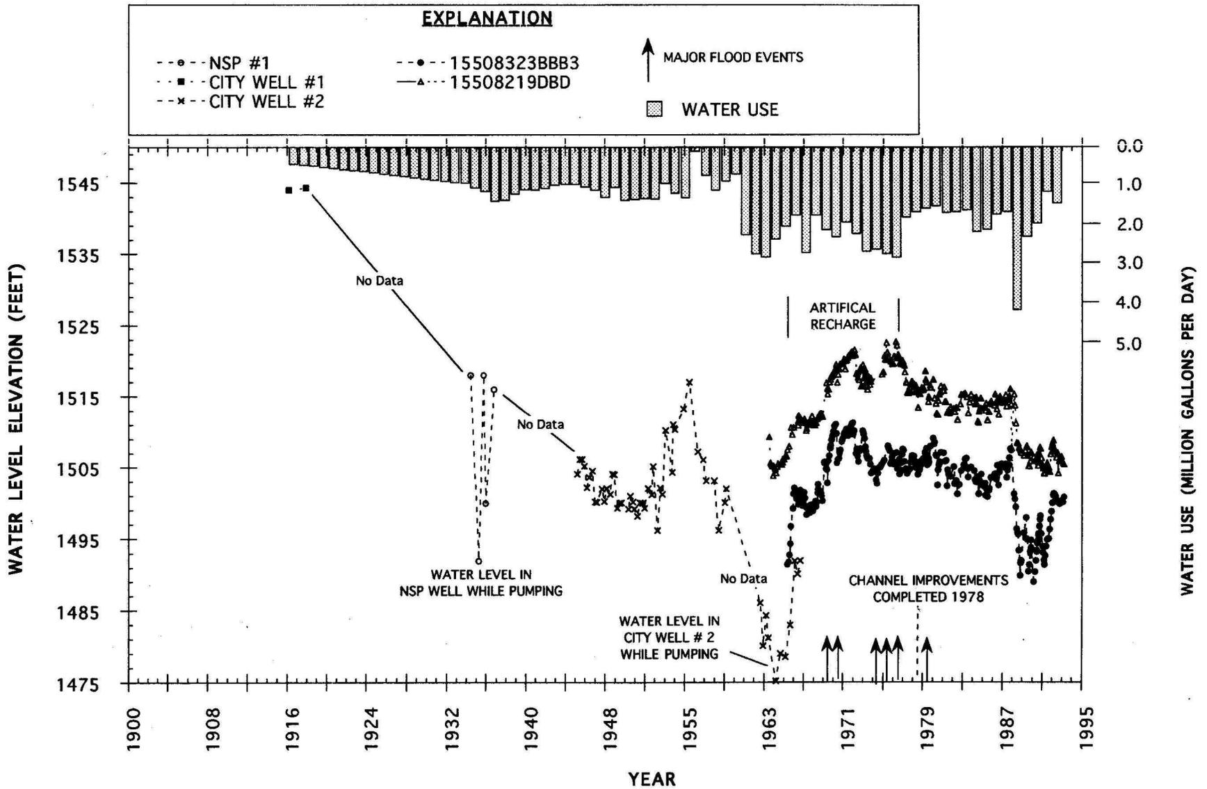
FIGURE 24. COMPARISON OF WATER LEVELS IN THE MINOT AQUIFER WITH WATER USE FROM THE MINOT AQUIFER (1916 - 1992)
