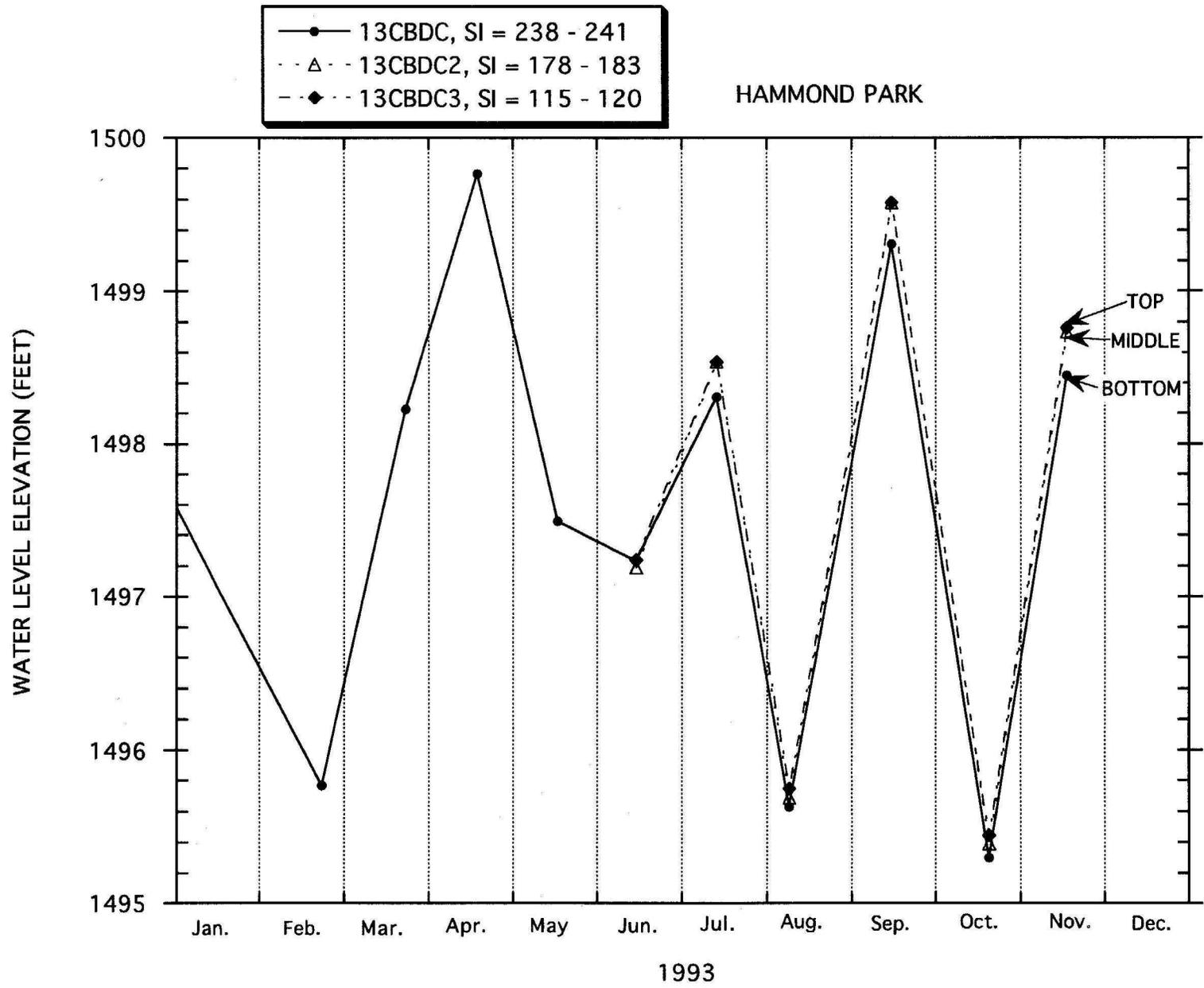
**FIGURE 27. HYDROGRAPHS OF WATER LEVELS FROM PIEZOMETER NEST 155-083-13CBDC SHOWING THE VERTICAL DISTRIBUTION OF WATER LEVELS IN THE MINOT AQUIFER.**
