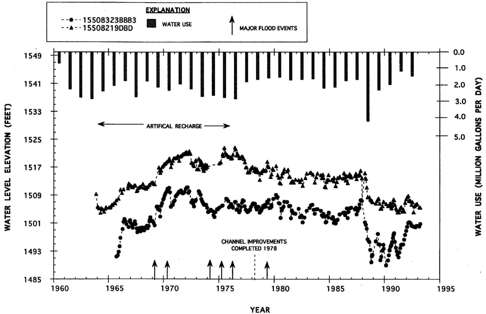
FIGURE 25. COMPARISON OF WATER LEVELS IN THE MINOT AQUIFER WITH WATER USE FROM THE MINOT AQUIFER (1964 - 1992)
