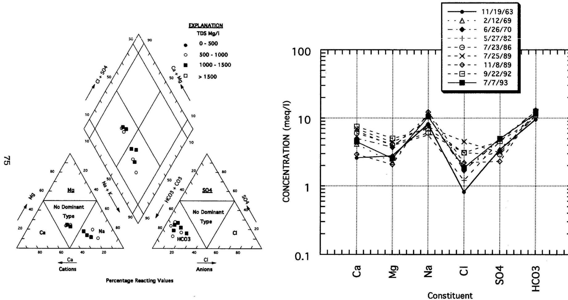
FIGURE 46. PIPER AND SCHOELLER DIAGRAMS SHOWING WATER QUALITY VARIATIONS WITH TIME, MINOT PRODUCTION WELL 12
