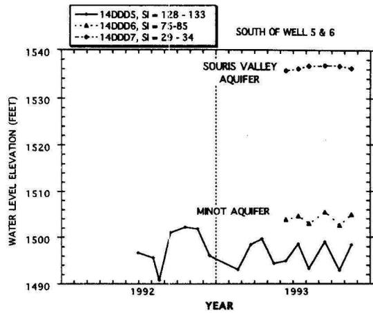
FIGURE 28. Hydrographs of water levels from piezometer nest 155-083-14DDD showing the vertical distribution of water levels in the Souris Valley and Minot aquifers.
