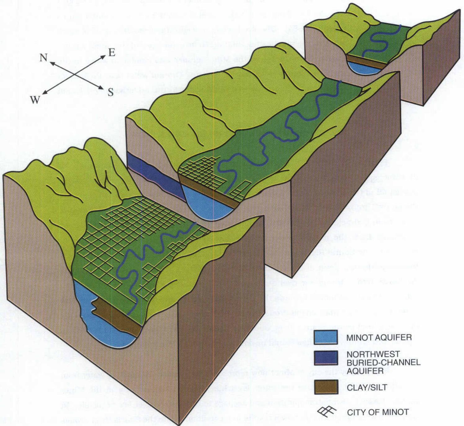
Figure 52. Schematic block diagram of the Souris River Valley in the Minot area illustrating the relationship of the major aquifers
