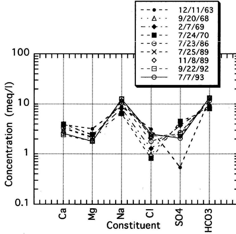
FIGURE 41. PIPER AND SCHOELLER DIAGRAMS SHOWING WATER QUALITY VARIATIONS WITH TIME, MINOT PRODUCTION WELL 16
