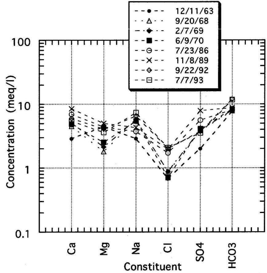
FIGURE 43. PIPER AND SCHOELLER DIAGRAMS SHOWING WATER QUALITY VARIATIONS WITH TIME, MINOT PRODUCTION WELL 15
