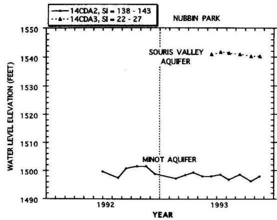
FIGURE 29. Hydrographs of water levels from piezometer nest 155-083-14CDA showing the vertical distribution of water levels in the Souris Valley and Minot aquifers.
