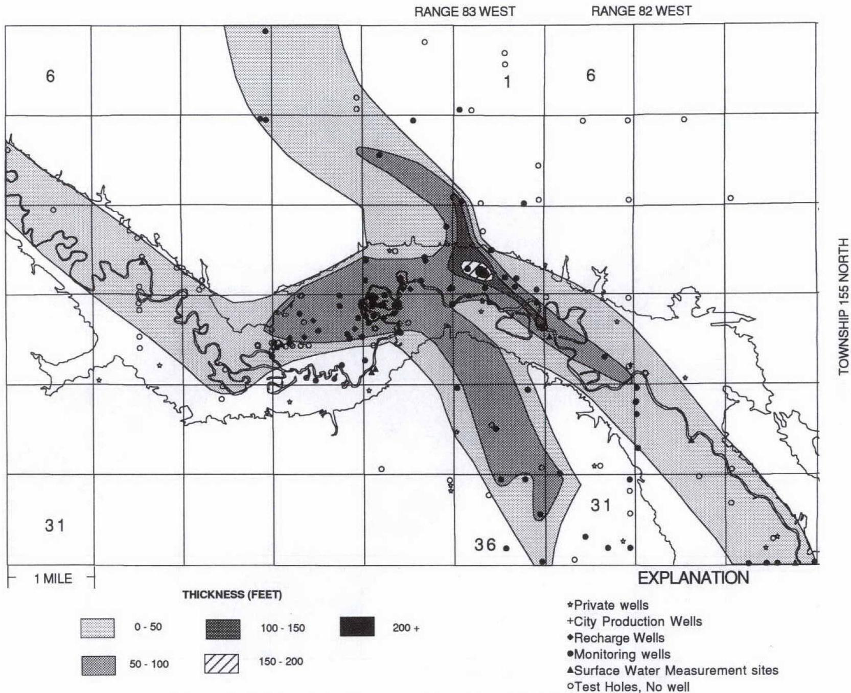
Figure 13. Saturated thickness of sand and gravel in the Minot area.
