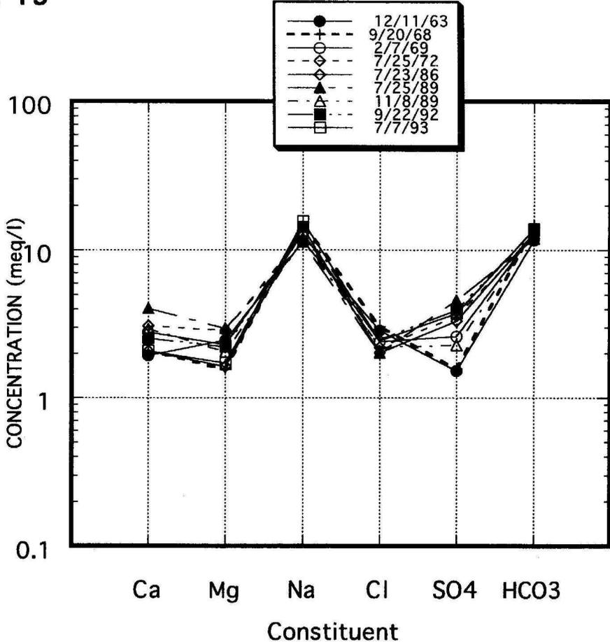
FIGURE 45. PIPER AND SCHOELLER DIAGRAMS SHOWING WATER QUALITY VARIATIONS WITH TIME, MINOT PRODUCTION WELL 13
