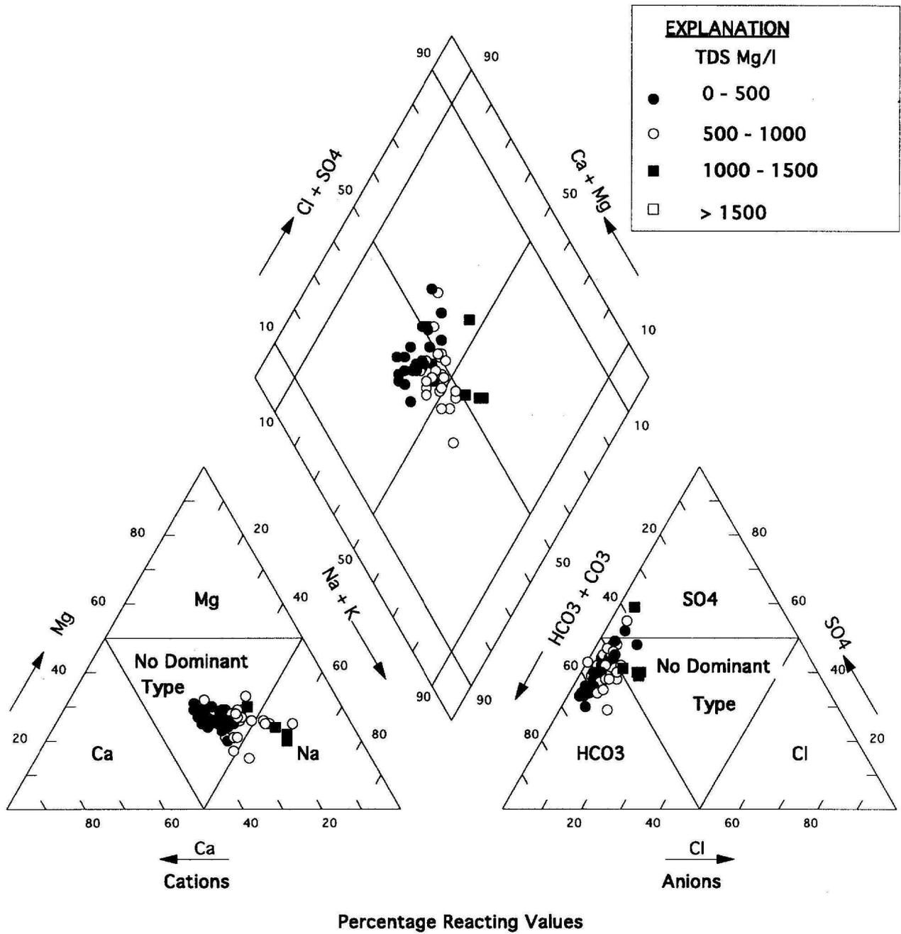
FIGURE 34. PIPER DIAGRAM SHOWING THE CHEMICAL QUALITY OF WATER FROM THE SOURIS RIVER ABOVE MINOT (1969 - 1992)
