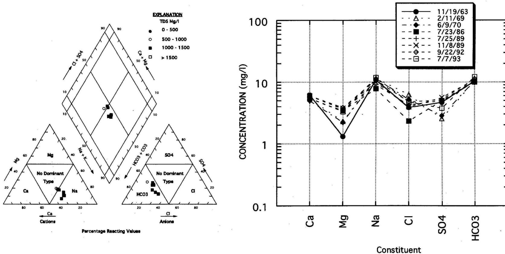
FIGURE 49. PIPER AND SCHOELLER DIAGRAMS SHOWING WATER QUALITY VARIATIONS WITH TIME, MINOT PRODUCTION WELL 6
