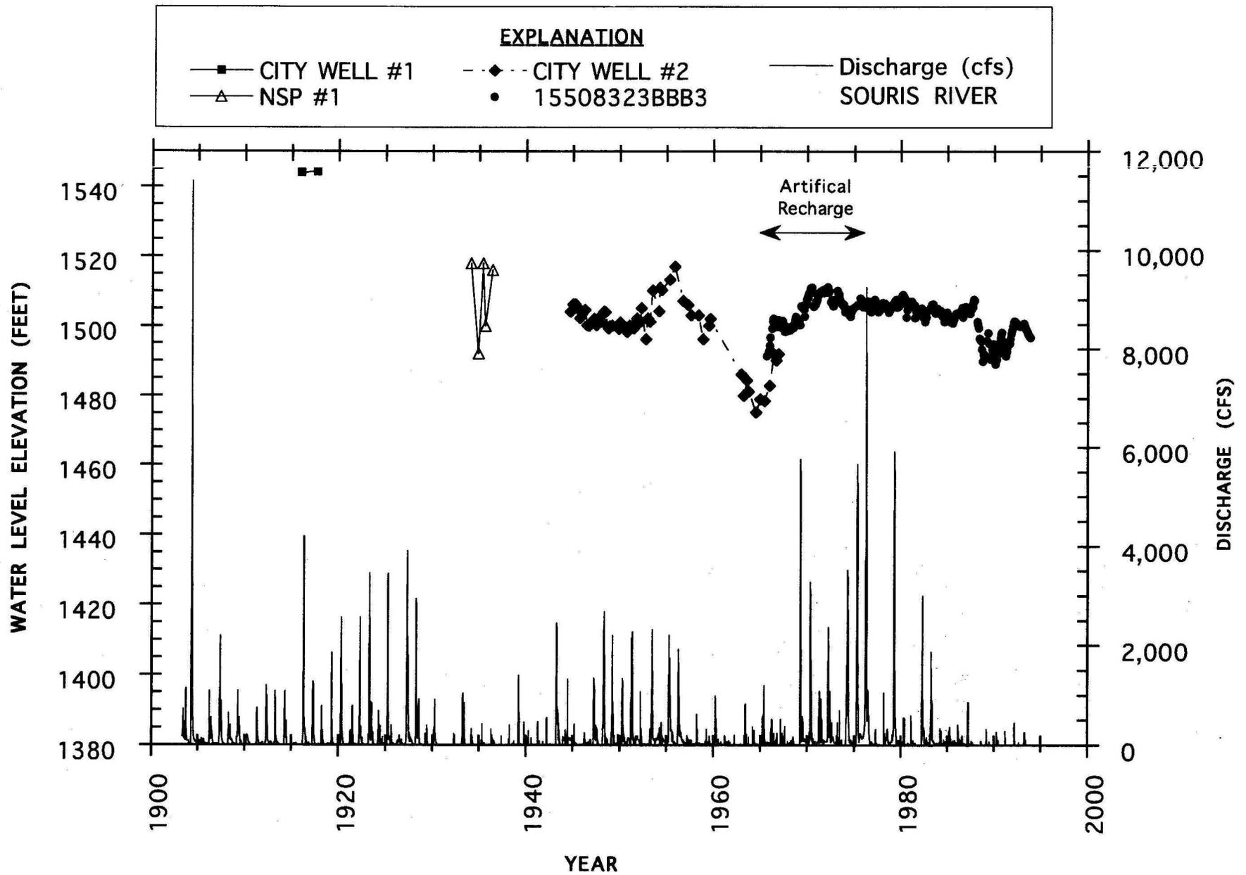
FIGURE 26. COMPARISON OF WATER LEVELS IN THE MINOT AQUIFER WITH DISCHARGE OF THE SOURIS RIVER ABOVE MINOT (1903 - 1992)
