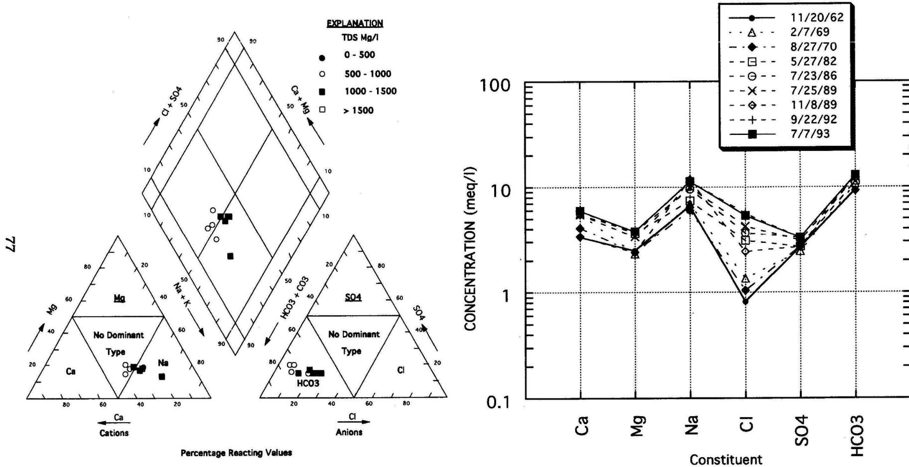
FIGURE 47. PIPER AND SCHOELLER DIAGRAMS SHOWING WATER QUALITY VARIATIONS WITH TIME, MINOT PRODUCTION WELL 11
