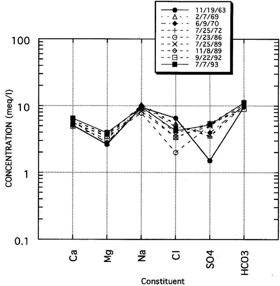
FIGURE 48. PIPER AND SCHOELLER DIAGRAMS SHOWING WATER QUALITY VARIATIONS WITH TIME, MINOT PRODUCTION WELL 5
