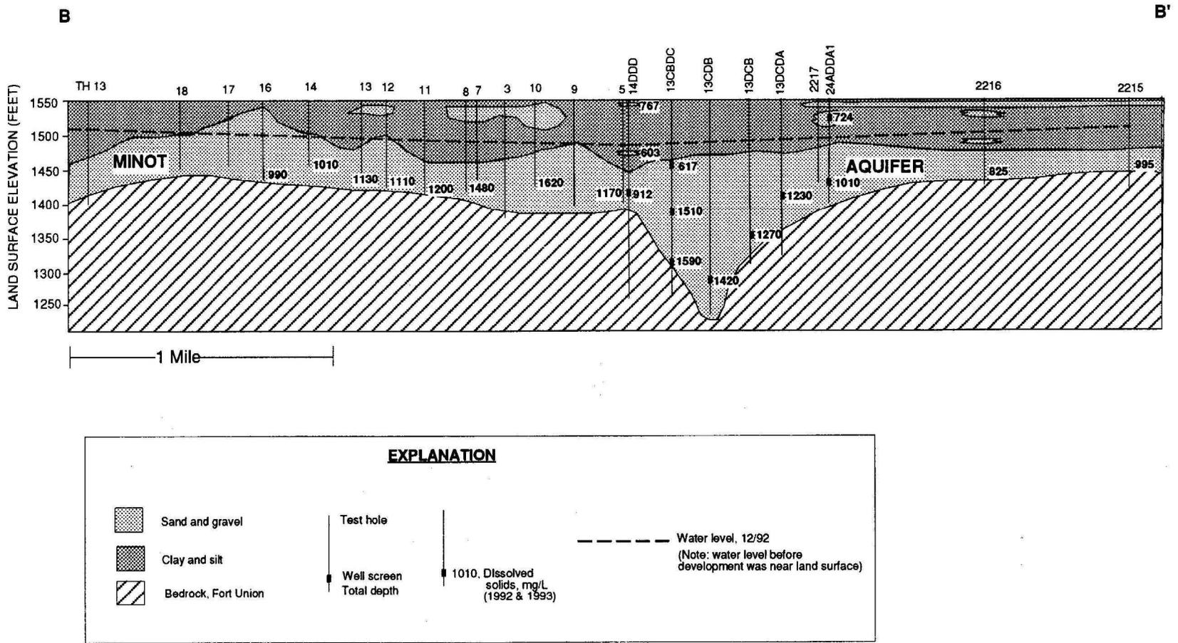
FIGURE 51. DISSOLVED SOLIDS CONCENTRATIONS AT SELECTED SITES IN THE MINOT AQUIFER ALONG HYDROGEOLOGIC SECTION B-B'
