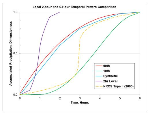
Figure 13.20: Comparison of final Local storm patterns to NRCS Type II temporal pattern
