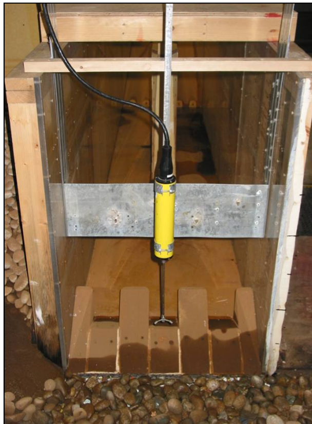
Figure A-50. —Looking upstream at stilling basin model with ADV probe and deflector installed near the end of basin.
