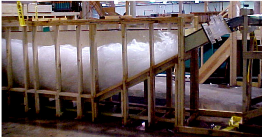
Figure A-49. —Looking through the plexiglass sidewall of the model operating at 40 percent gate opening.
