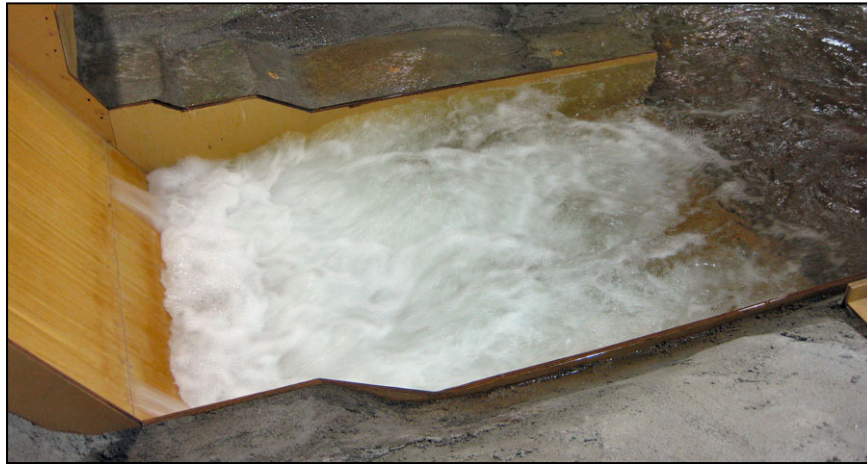
Figure 41. —This figure shows a hydraulic jump occurring in a 1:48-scale model of a type V stilling basin for a spillway. The operating condition equates to a prototype discharge of 60,000 ft 3 /s. The 242-foot wide stilling basin has an 0.8:1 slope for the upstream 178.7-foot length and is horizontal for the downstream 146.8-foot length. The stilling basin has a 15-foot high solid end sill. The figure most closely depicts the condition discussed in case C where the upstream toe of the hydraulic jump occurs on the slope and the downstream end of the jump is at the junction of the slope and the horizontal apron (for this example, where the break in floor slope goes from 0.8:1 to horizontal).
