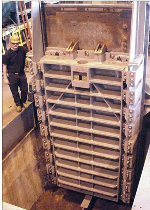
Figure 114. —Fixed-wheel gate measuring 16 feet wide by 26 feet high. Photo courtesy of Rodney Hunt Corporation.
