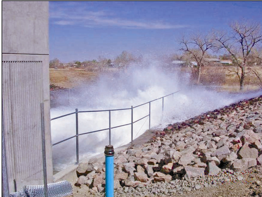
Figure A-100. —View looking downstream shown the right fixed-cone valve discharging at 35 percent opening (150 ft 3 /s).
