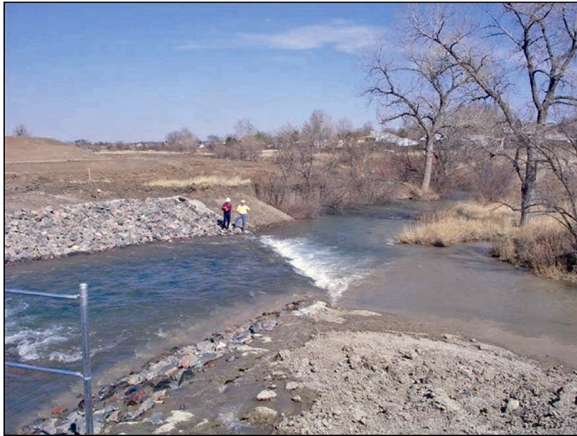
Figure A-99. —View looking downstream at the outfall channel during testing of one of the fixed-cone valves at 35 percent opening (147 ft 3 /s).
