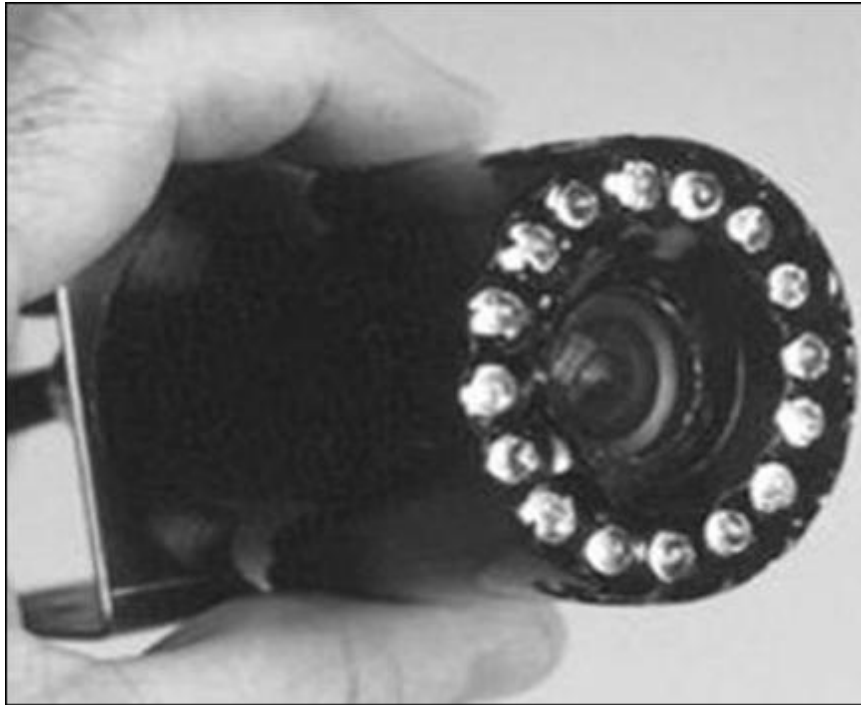
Figure A-105. —Subsea mini video camera used to inspect small pipes. Note the 16 LED light sources surrounding lens.
