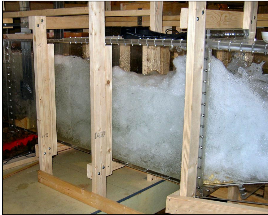
Figure 17. —The Froude number for the discharge in this model study is greater than 10.0. Note the rough water surface with strong waves downstream from the jump.
