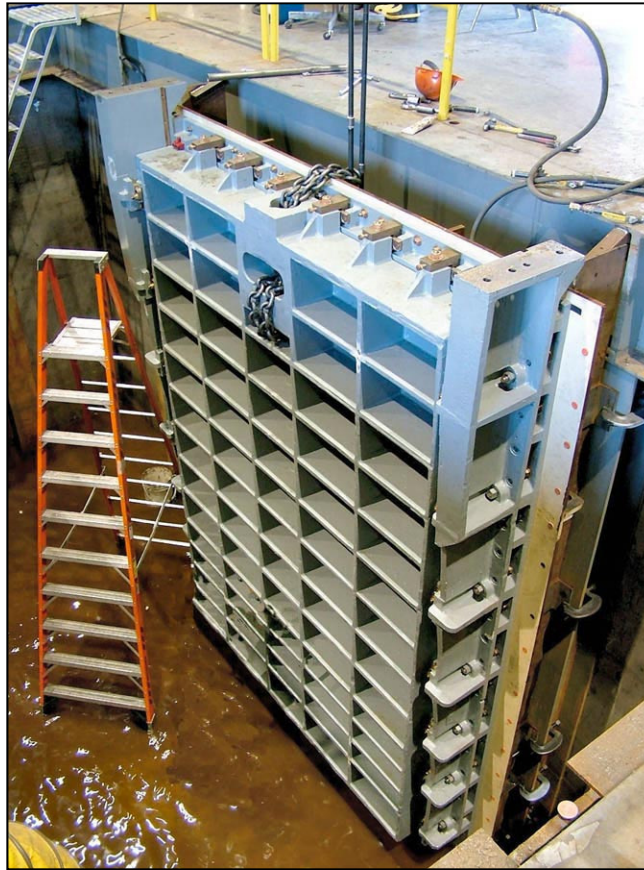
Figure 105. —Shop testing of cast-iron slide gate. Photo courtesy of Rodney Hunt Corporation.
