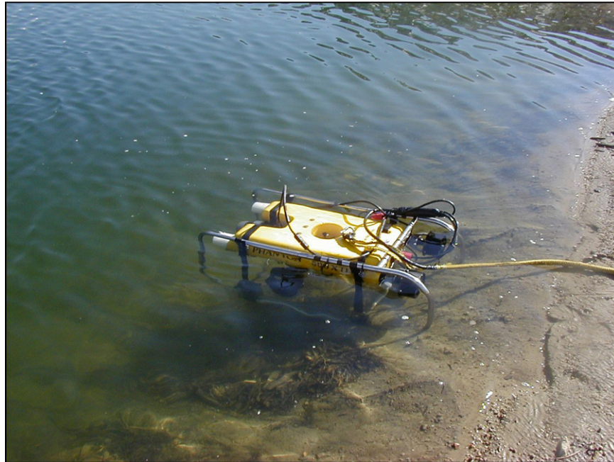
Figure 159. —An observation-class ROV entering the water to begin an inspection.
