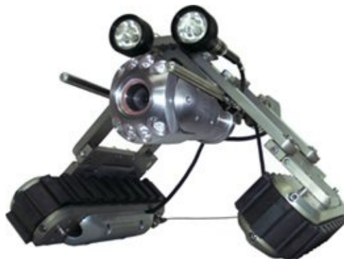
Figure 160. —A camera-crawler used for CCTV inspection.
