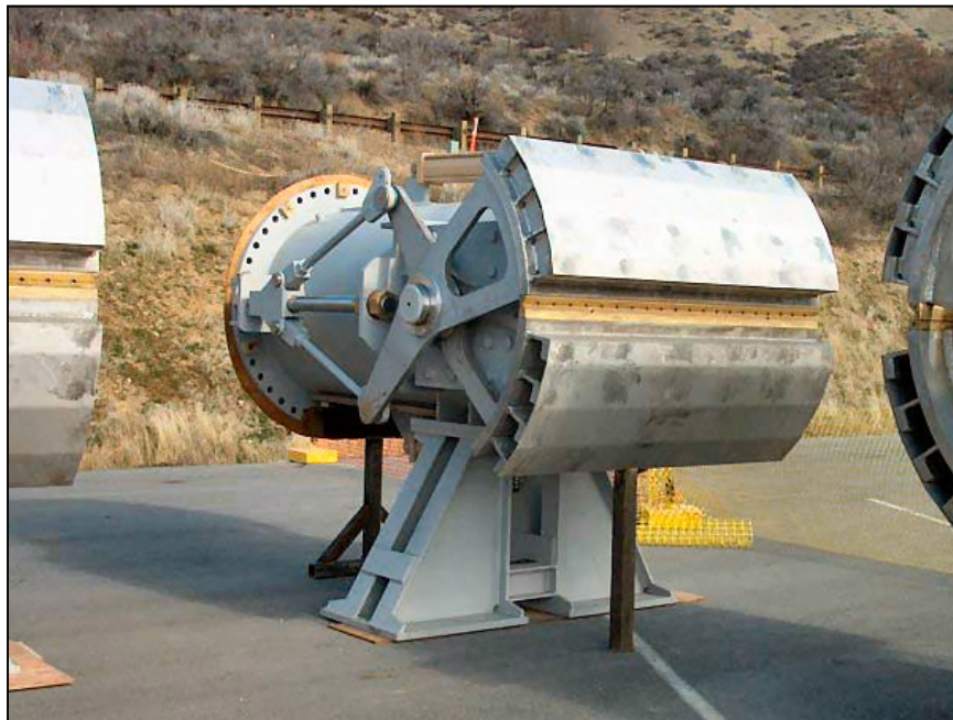
Figure 108. —48-inch diameter clamshell gate before installation.
