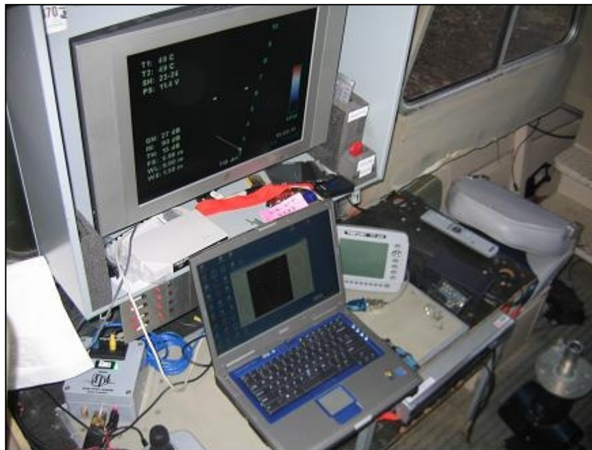
Figure 162. —Interior of a USACE boat equipped for surface deployment of an acoustical imaging system.
