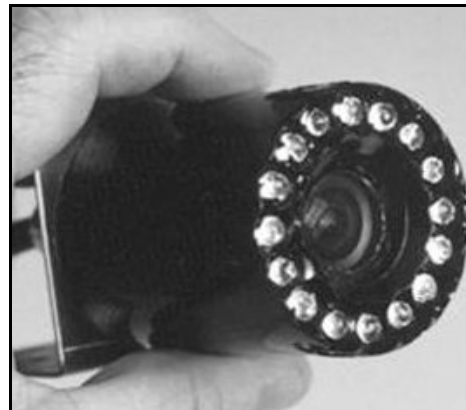
Figure 131. —A small color video camera used for CCTV inspection.
