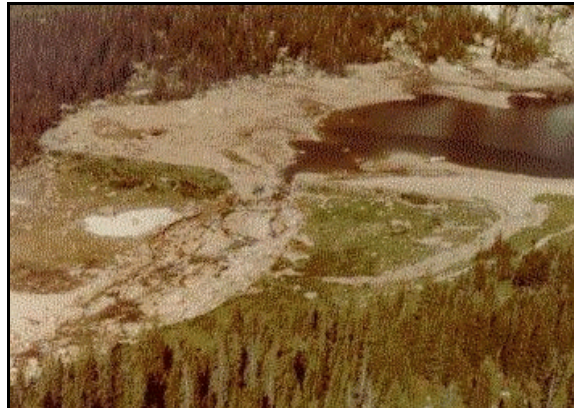
Figure B-46. —Aerial view of the breached Lawn Lake Dam and downstream floodplain.
