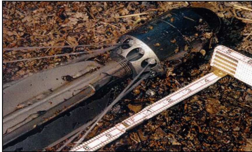
Figure 133. —Pressure washing cleaning head.
