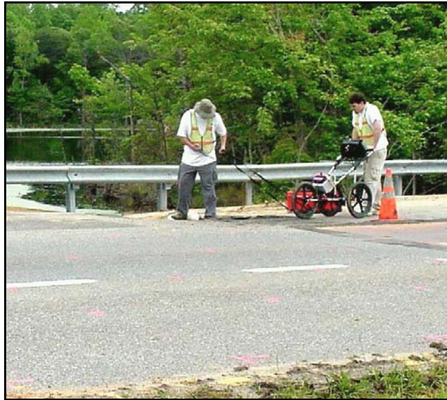
Figure B-30. —Ground penetrating radar investigations were performed from the embankment dam crest.
