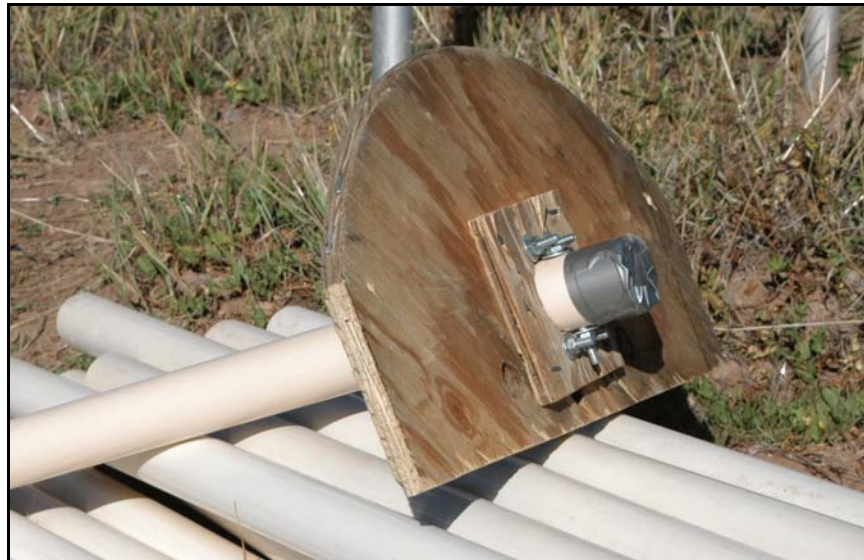
Figure 161. —A horseshoe shaped template used for checking irregularities in a conduit. The template is attached to the CCTV camera-crawler.
