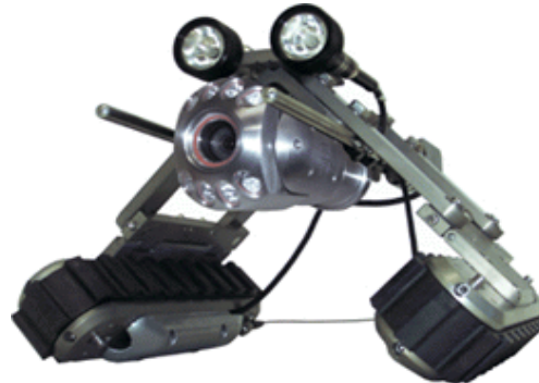
Figure 129. —Camera-crawler used for CCTV inspection of conduits. Photo courtesy of Inuktun Services, Ltd.
