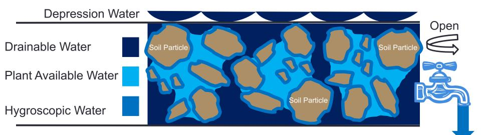
As conditions allow, subsurface drains can be opened to drain the soil profile and surface depression water in preparation for a spring flood event.
