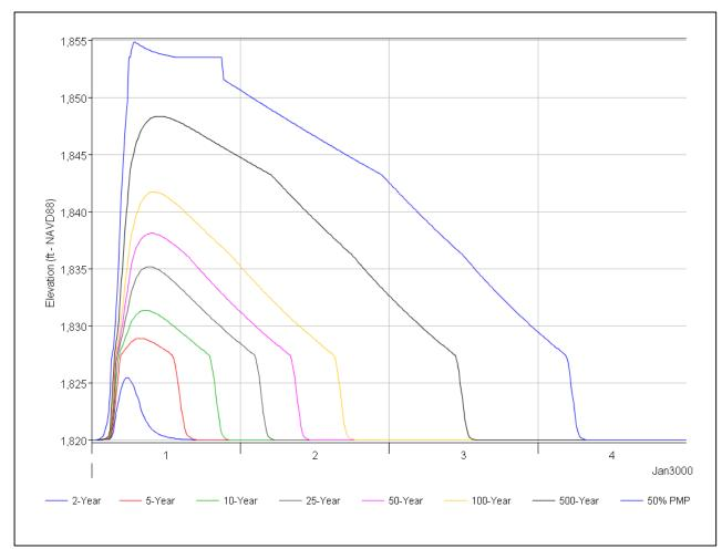
Figure 8. Reservoir Elevation for Frequency Events.
