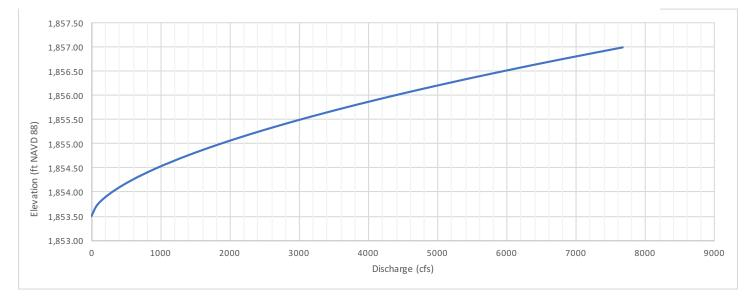
Figure 7. Emergency Spillway Elevation-Discharge Curve.
