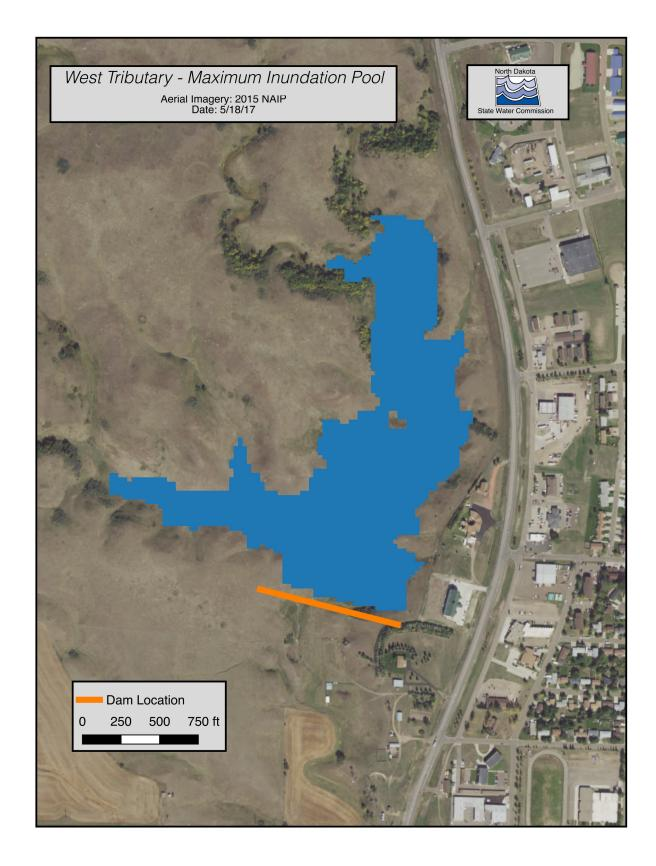
Figure 4. Maximum pool inundation.
