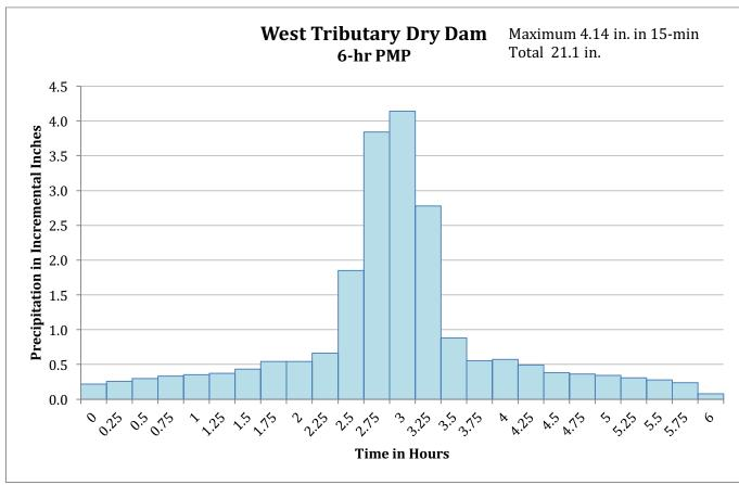
Figure 2. Balanced PMP Hyetograph.
