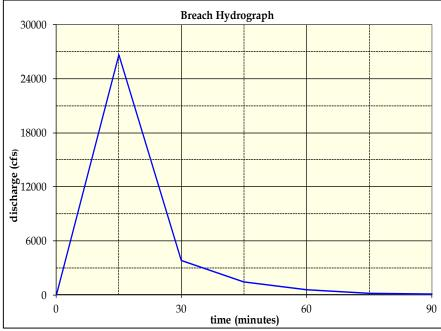
Figure 9. Calculated Breach Hydrograph.
