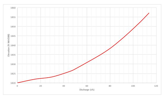
Figure 6. Principal Spillway Elevation-Discharge Curve.
