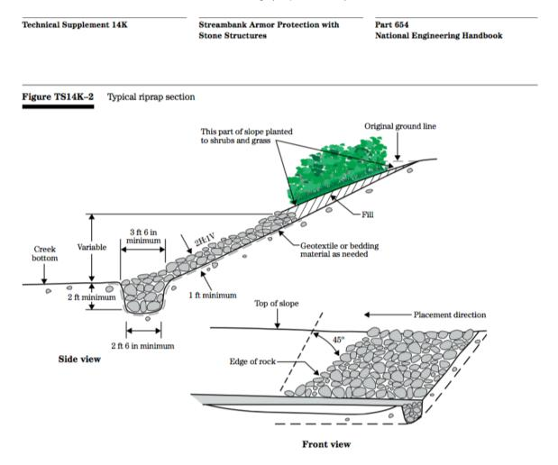
Figure 6. Typical riprap section (NRCS, 2007)
