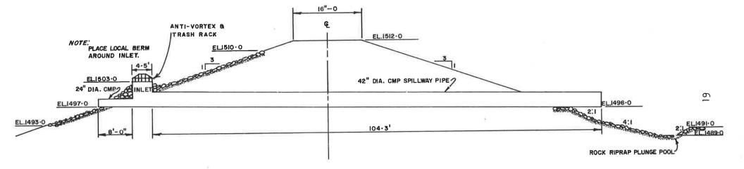
TYPICAL CROSS SECTION OF DAM AT MAIN SPILLWAY
