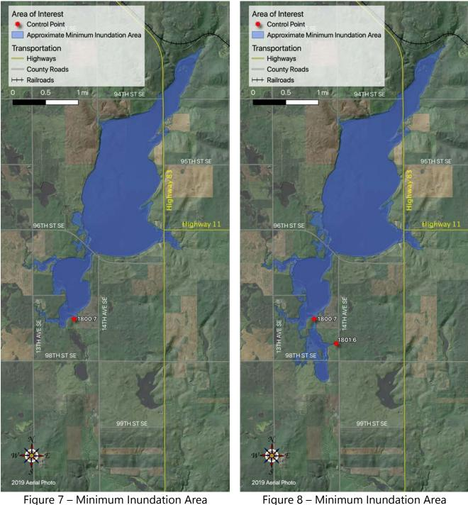
Figure 8 – Minimum Inundation Area Corresponding to Control Point 2
