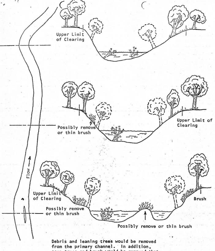
Debris and leaning trees would be removed from the primary channel. In addition, some trees and brush would be removed that are on eroded banks or very low on the bank in the primary channel. The upper limit of clearing is the top of the primary bank.
