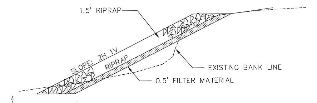
Figure 2 Typical Section of Protected Streambank
