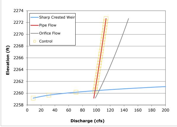
Figure 5. Principal Spillway Rating Curve
