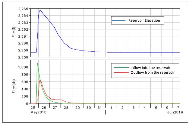
Figure 9. Pool elevation, inflow, and outflow for the  $P_{100}$  case.
