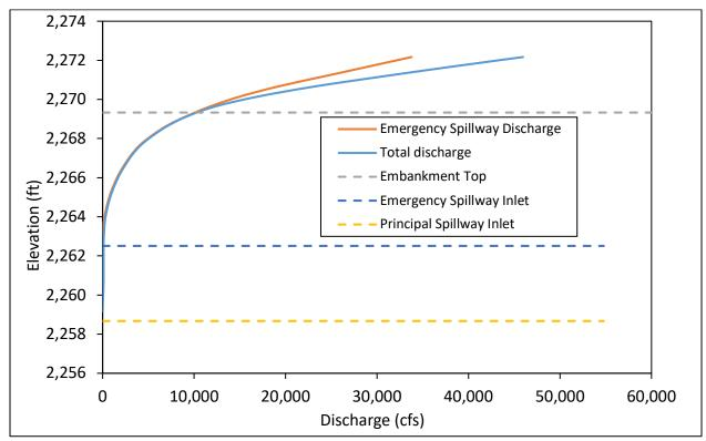
**Figure 8.** Total discharge (combination of principal spillway, emergency spillway, and overtopping) and emergency spillway rating curves for given pool elevations.
