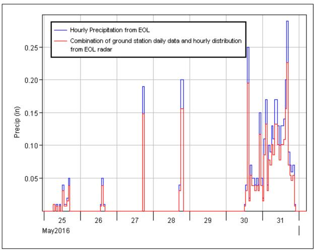
**Figure 3**. Hourly precipitation generated from the combination of ground station daily data and hourly distribution from radar (red line), and hourly precipitation from EOL (blue line).
