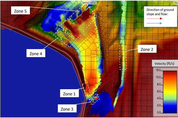
Figure 10. Discharge velocities downstream of the emergency spillway.
