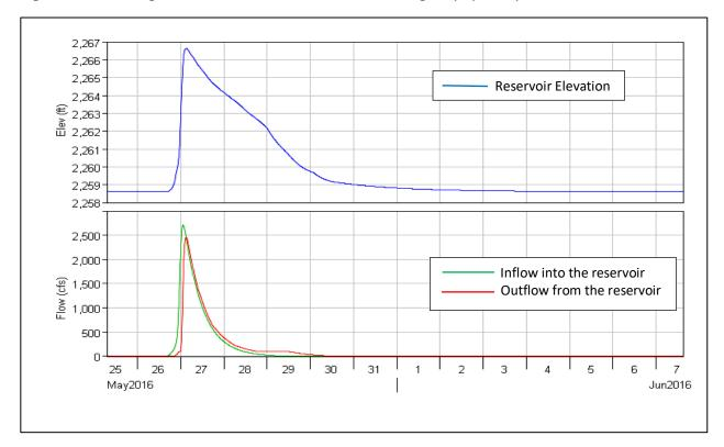
Figure 11. Pool elevation, inflow, and outflow for the 0.4 PMP case.
