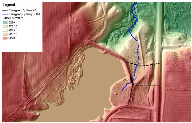
**Figure 6**. Cross sections for HEC-RAS simulation (black dashed lines represent cross sections and the blue line represents the flow path along the emergency spillway).
