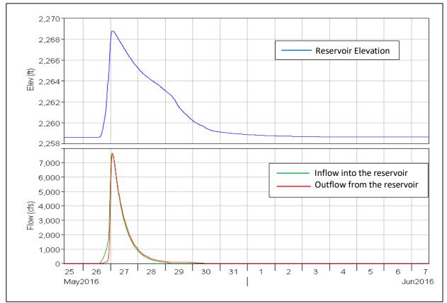
Figure 13. Pool elevation, inflow, and outflow for the PMP case.
