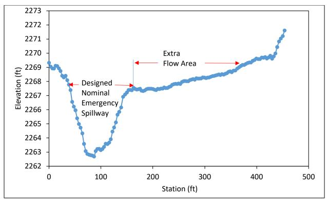
Figure 7. Profile of emergency spillway crest.
