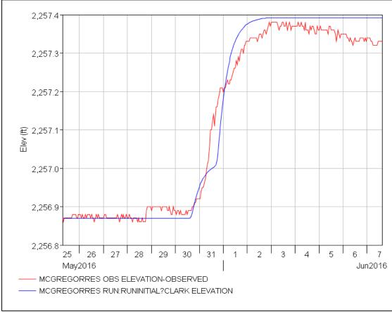
**Figure 4.** Agreement between observed and simulated pool elevation time series for calibration.
