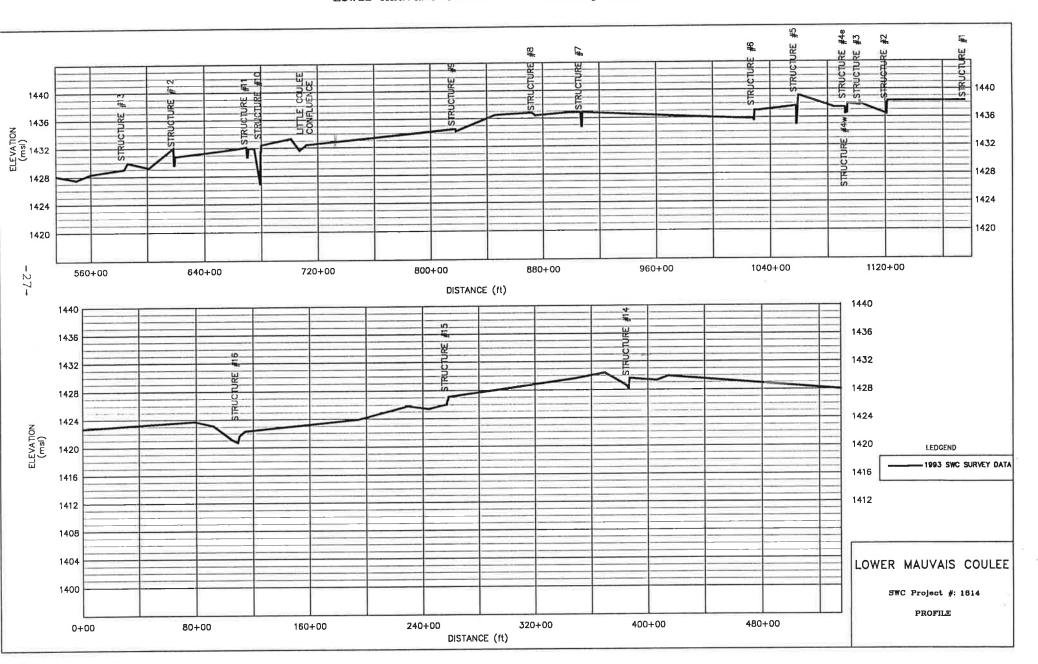
Figure 5 - Channel Profile of Lower Mauvais Coulee for Existing Conditions
