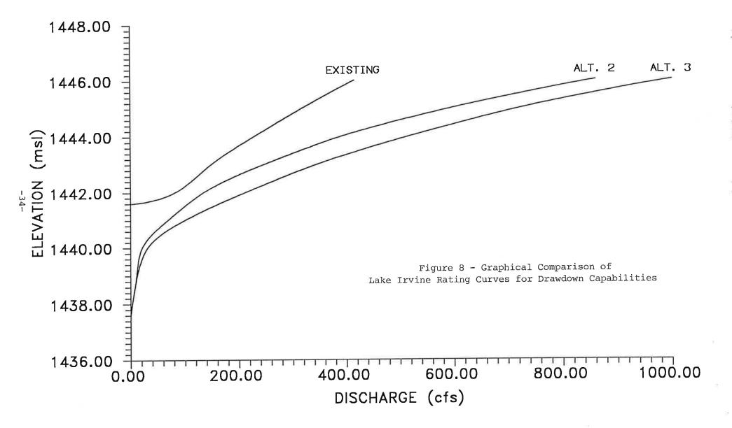
Two with the stop logs removed from the control structure, and for Alternative Three with the stop logs removed from the control structure.
