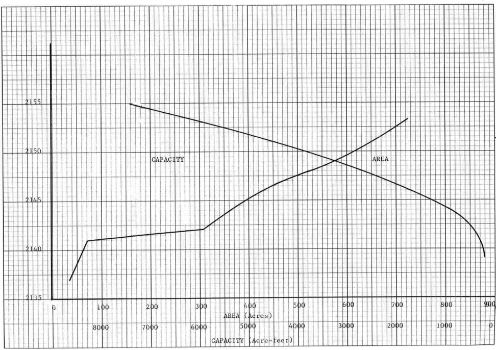
FIGURE 3 - AREA - CAPACITY CURVE FOR ROST-SCHOOL SECTION LAKE DAM
