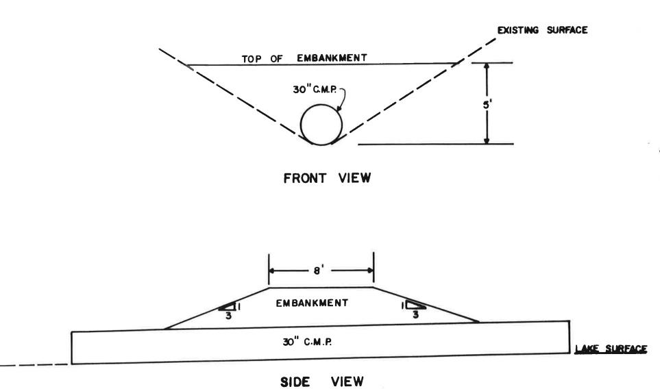
FIGURE II-TYPICAL CONTROL STRUCTURE NOT TO SCALE
