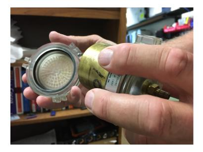
Figure 16. Acrylic disc used for Ks and  $K(\psi/\theta)$  measurements. Disc was overlain by a 0.11 mm thin porous nylon membrane.
