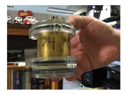
Figure 15. Tempe cell assembly used to measure Ks and  $K(\psi/\theta)$ .
