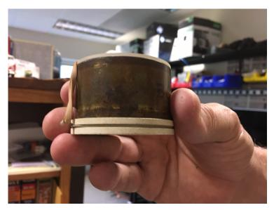
Figure. 4. Sample-plate assembly used for measurement of soil water-retention curves.
