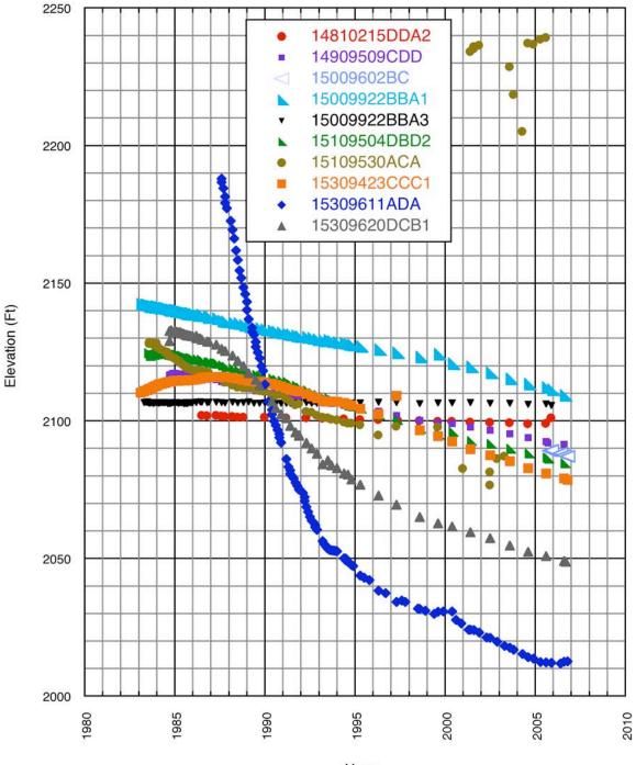
Figure 8 -- Hydrograph showing the historical water-level fluctuations in 10 observation wells installed in the Fox Hills aquifer
