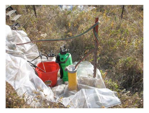
Photo 4. Purging a well using a gas squeeze pump.
