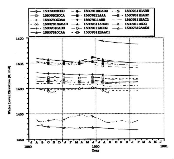
Figure 12 - Hydrograph of water-level elevations observed in the eastern terrace unit of the Souris Valley aquifer.
