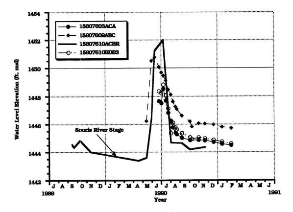
Figure 14 - Hydrograph comparing the water-level elevations in the deeper channel unit of the Souris Valley aquifer with the Souris River stage.
