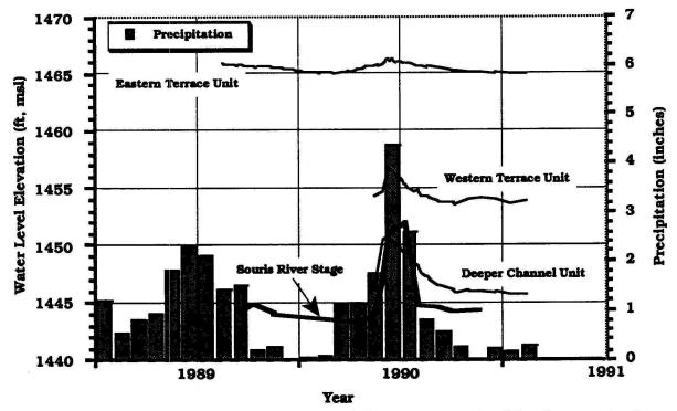
Figure 13 - Hydrograph comparing water-level elevations in each of the three units of the Souris Valley aquifer with the Souris River stage and recorded precipitation.
