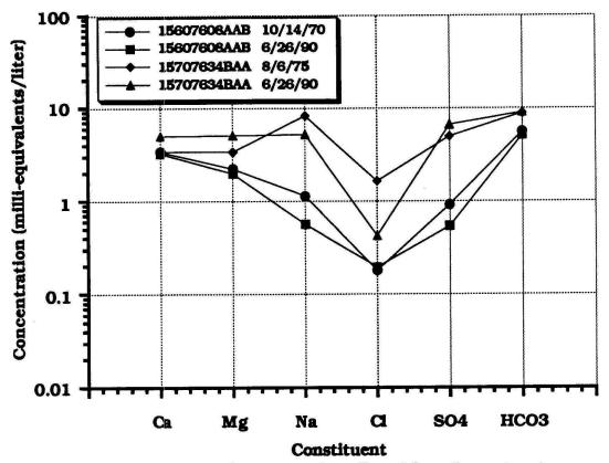
Figure 17 - Schoeller diagram of water samples collected from the western terrace unit of the Souris Valley aquifer.
