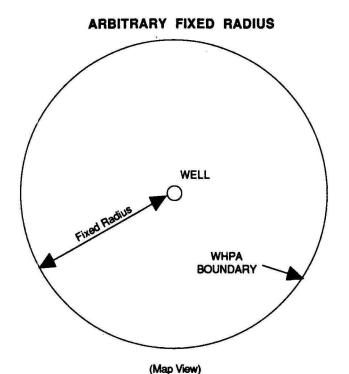
Figure 19 - Arbitrary Fixed Radius method of Wellhead Protection Area Delineation.
