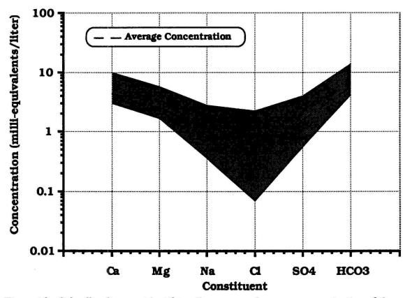
Figure 16 - Schoeller diagram identifying the range and average concentration of the major cations and anions from wells completed in the eastern terrace unit with the exception of wells completed along the southern boundary.
