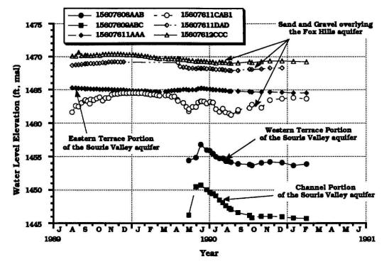
Figure 8 - Hydrograph comparing the relationship between the water levels observed in the sand and gravel overlying the Fox Hills aquifer with the water levels observed in the Souris Valley aquifer.
