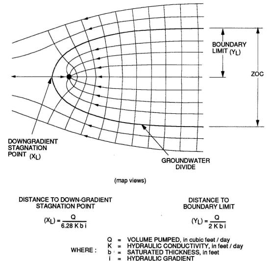
Figure 21 - Zone of Contribution method of Wellhead Protection Area delineation (modified from Todd, 1980).
