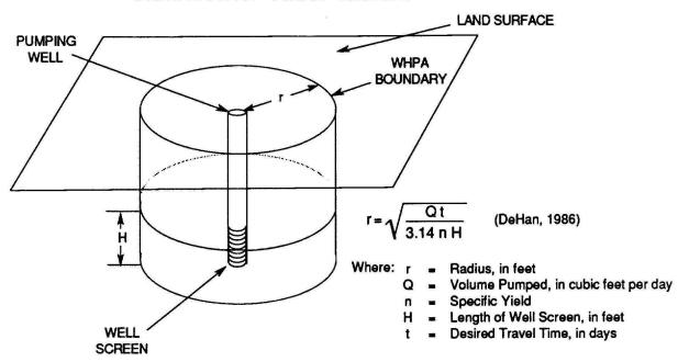
Figure 20 - Calculated Fixed Radius method of Wellhead Protection Area delineation.
