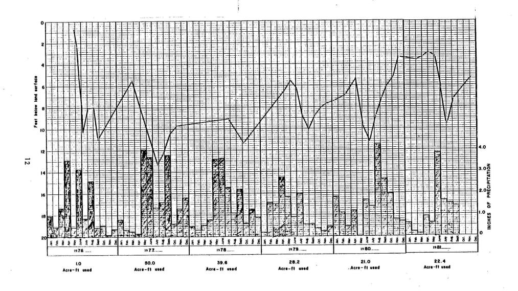
FIG. 5- Hydrograph for 155-81-11 ccd
