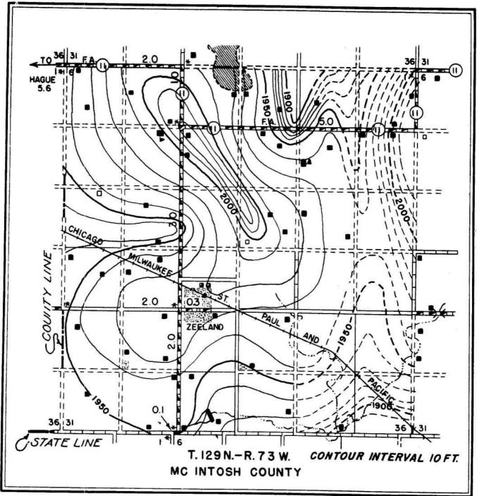
FIG. 2- WATER-TABLE CONTOUR MAP (BASED ON SEA-LEVEL DATUM)
