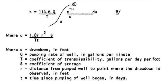
There are several methods of computing the coefficients of storage and transmissibility from this equation and from approximate expressions derived from it. The coefficients of transmissibility and storage were computed by several methods in order to ascertain whether any boundaries or marked changes in the character of the aquifer are present near the well which might be recognized by the nature of the results obtained.
