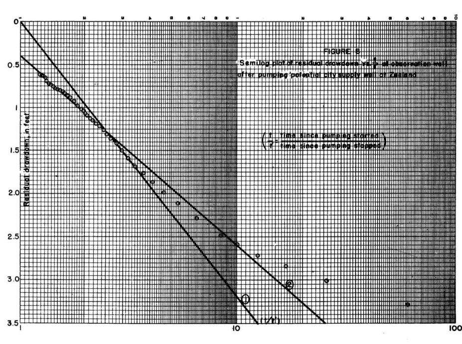
The coefficient of transmissibility is calculated from the equation where
