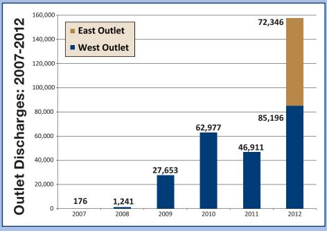
By starting the West Devils Lake Outlet a month earlier than normal, and with the operation of the newly constructed East Devils Lake Outlet, the State Water Commission was able to remove a record amount of water from Devils Lake in 2012. Water removed by the outlets accounted for about 1 foot, of the over 2 feet that Devils Lake dropped in 2012.
