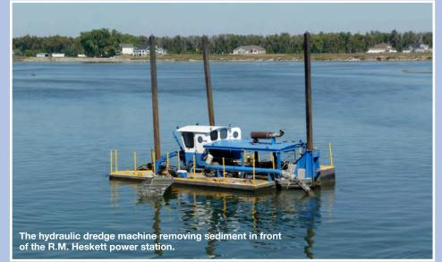
Water and sediment are pumped into one of two upland disposal sites. The disposal sites are designed to have the sediment settle out, and for some of the water to return back into the river via gravity flow.
