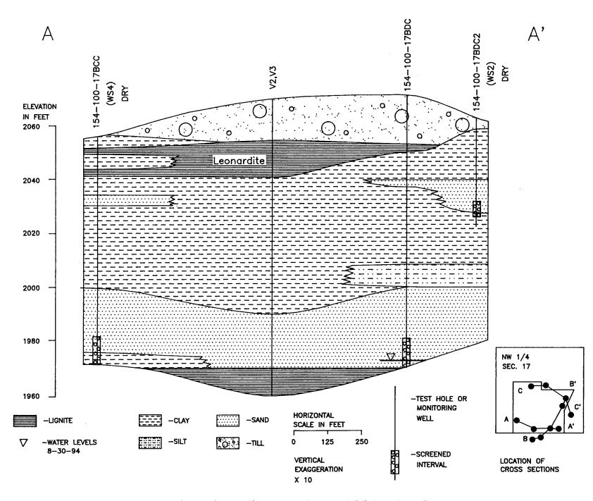
Figure 5. Geohydrologic section A-A' in the Williston landfill.
