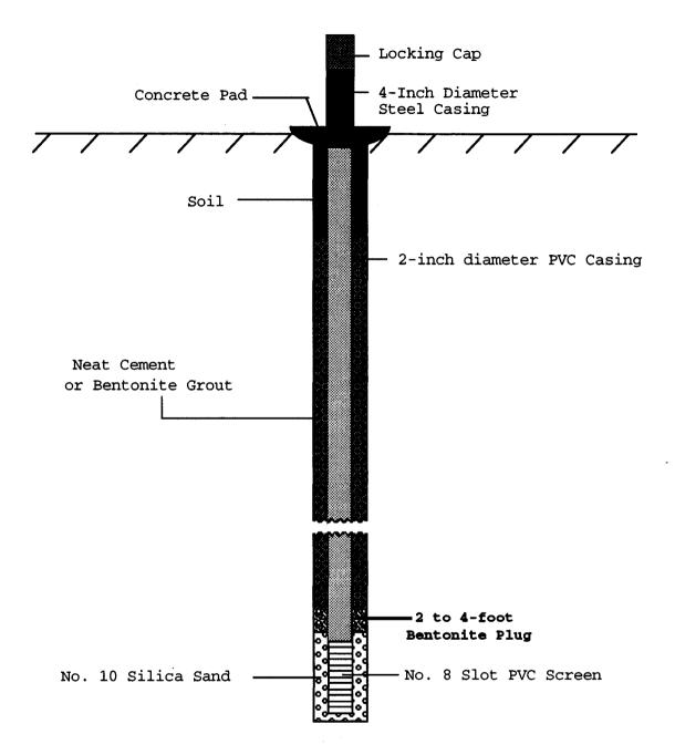
Figure 2. Construction design used for monitoring wells installed at the Williston landfill.
