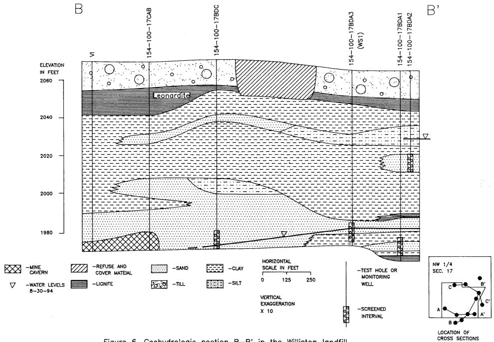
Figure 6. Geohydrologic section B-B' in the Williston landfill.
