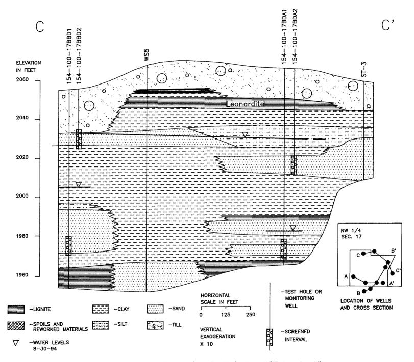
Figure 7. Geohydrologic section C-C' in the Williston landfill.
