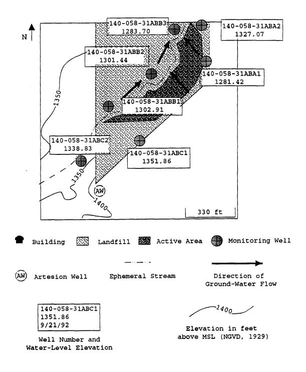
Figure 5. Location of monitoring wells and ground-water flow at the Valley City landfill.
