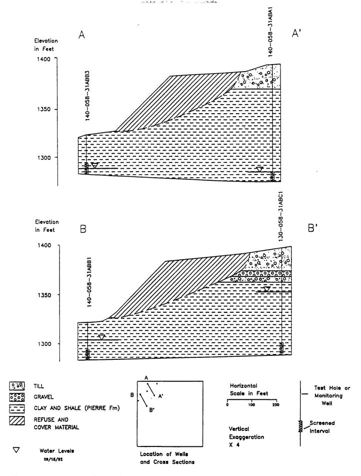
Figure 6. Geohydrologic sections A-A' and B-B' in the Valley City Landfill
