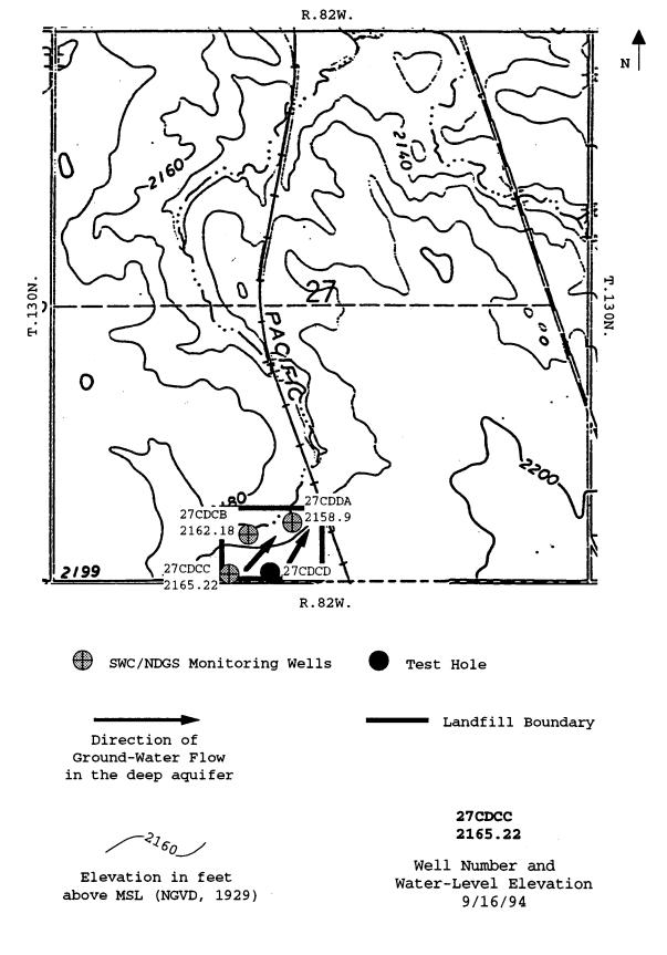
Figure 5. Location of monitoring wells and the direction of ground-water flow.
