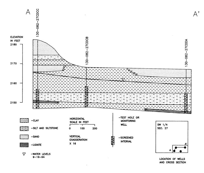
Figure 6. Geohydrologic section A-A' in the Selfridge landfill.
