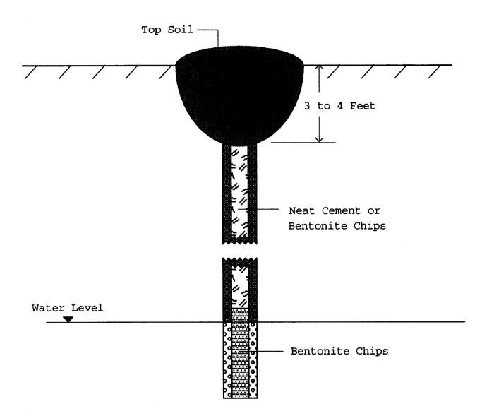
Figure 3. Monitoring well abandonment procedures.
