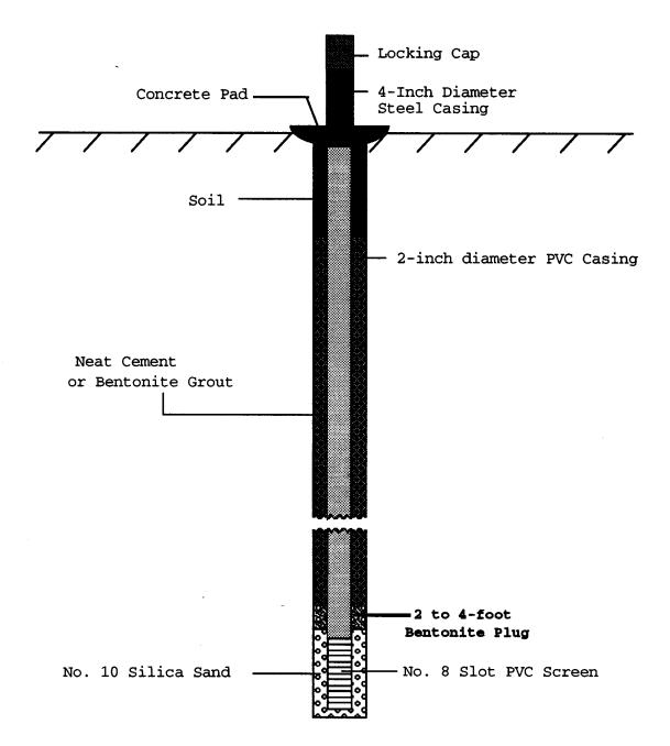
Figure 2. Construction design used for monitoring wells installed at the Selfridge landfill.
