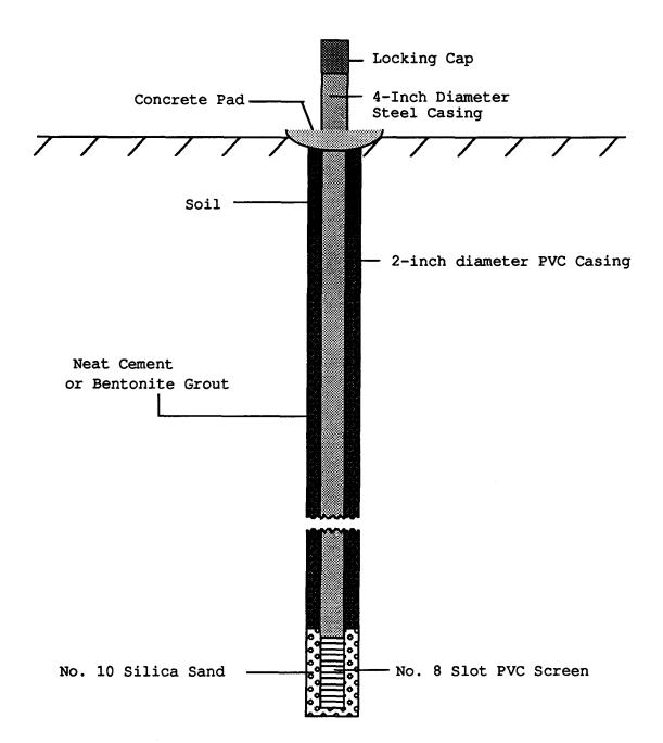
Figure 2. Construction design used for monitoring wells installed at the Rolla landfill.
