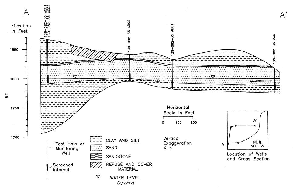
Figure 6. Geohydrologic section A-A' in the Mandan landfill
