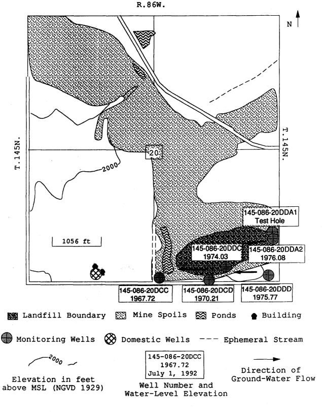
Figure 4. Location of monitoring wells and the direction of ground-water flow at the Devils Lake landfill.
