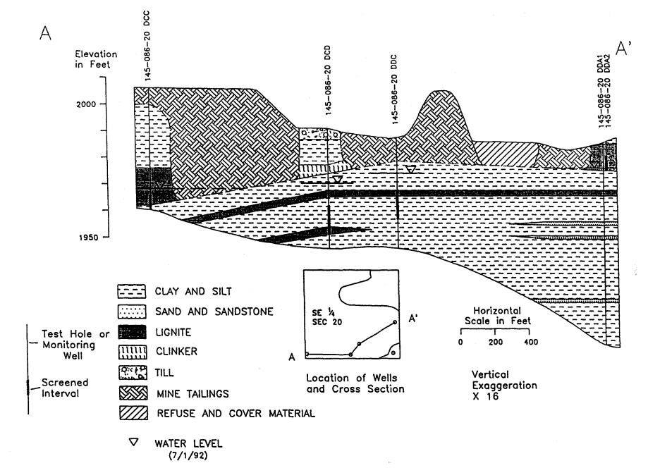
Figure 6. Geohydrologic section A-A' in the Hazen landfill
