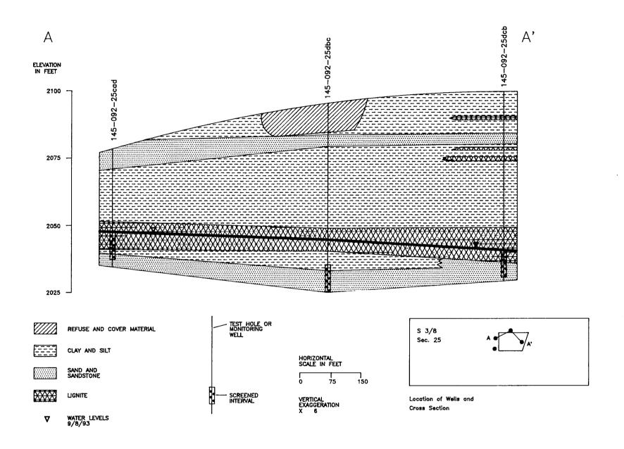
Figure 6. Geohydrologic section A—A' in the Halliday landfill.
