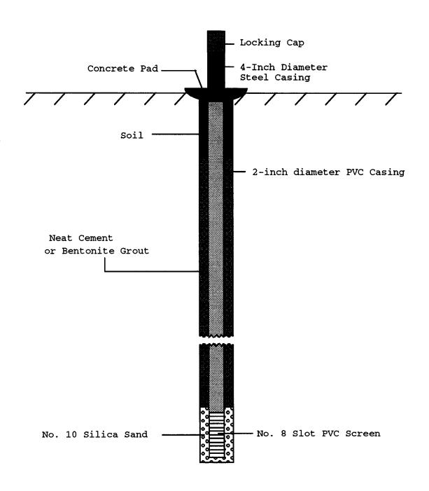
Figure 2. Construction design used for monitoring wells installed at the Halliday landfill.
