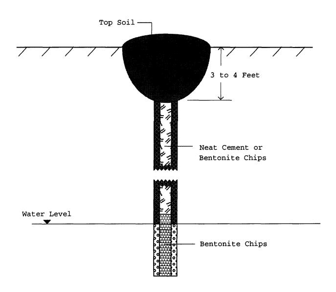
Figure 3. Monitoring well abandonment procedures.
