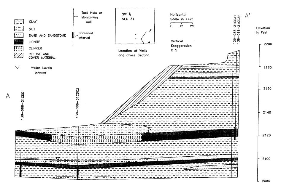
Figure 5. Geohydrologic section A-A' in the Glen Ullin landfill
