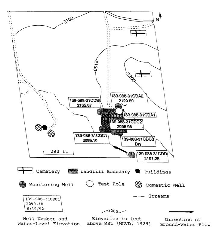
Figure 4. Location of monitoring wells and the direction of ground-water flow.
