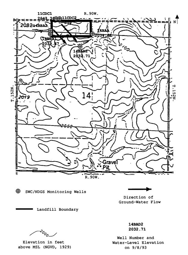
Figure 5. Location of monitoring wells at the Geving Sanitation landfill.
