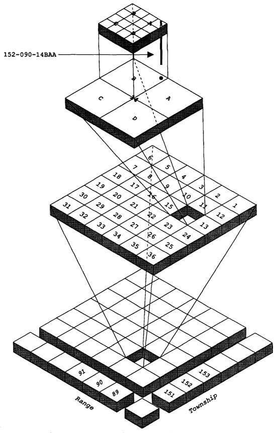
Figure 4. Location-numbering system for the Geving landfill.
