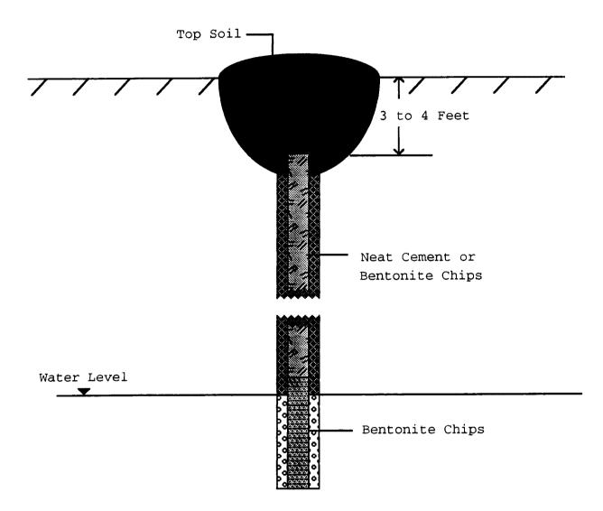
Figure 3. Monitoring well abandonment procedure.
