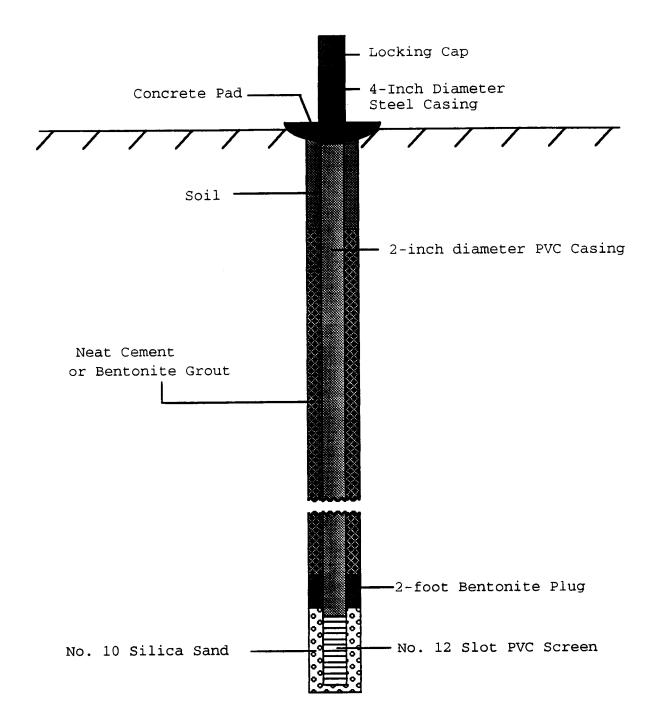
Figure 2. Construction design used for monitoring wells installed at the Gahner landfill.
