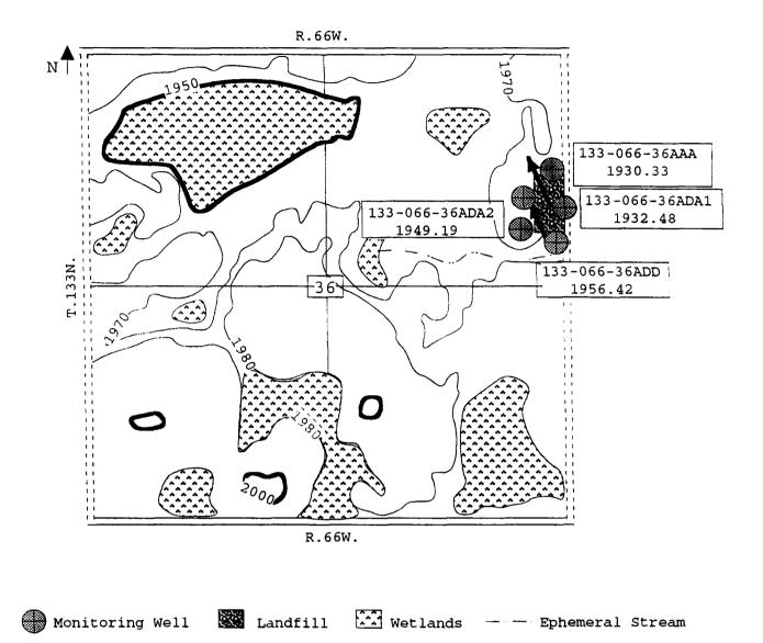
Figure 5. Location of monitoring wells and the direction of ground-water flow in the till aquifer.
