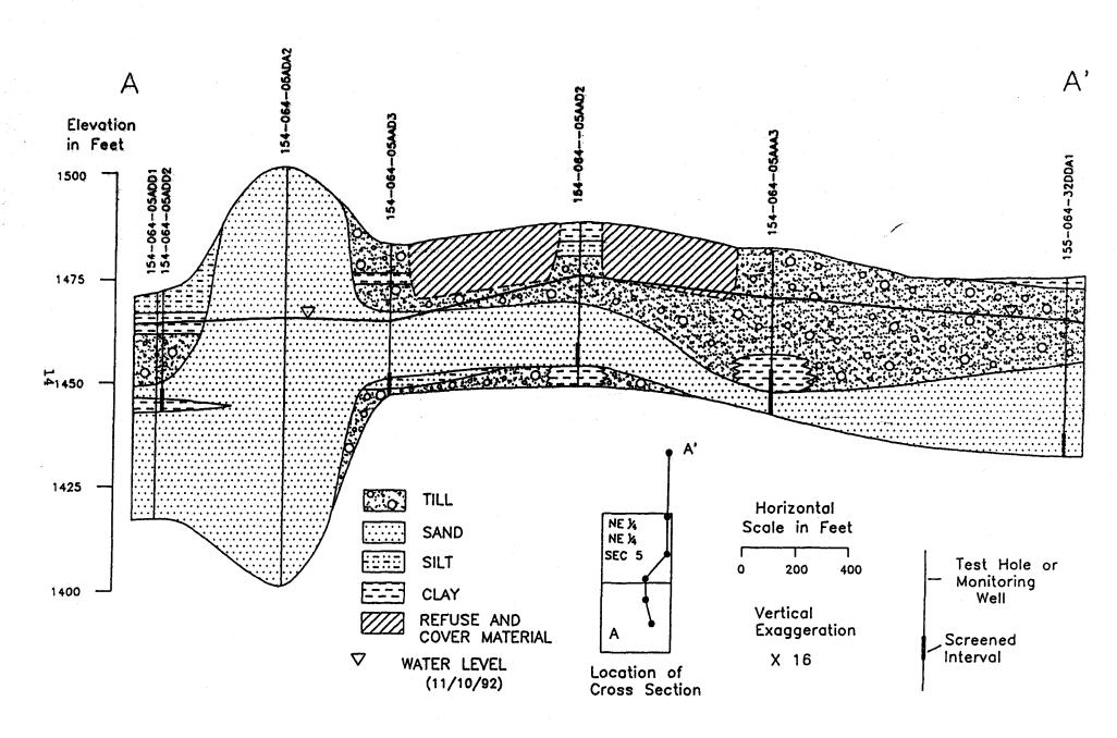
Figure 5. Geohydrologic section A-A' in the Devils Lake landfill
