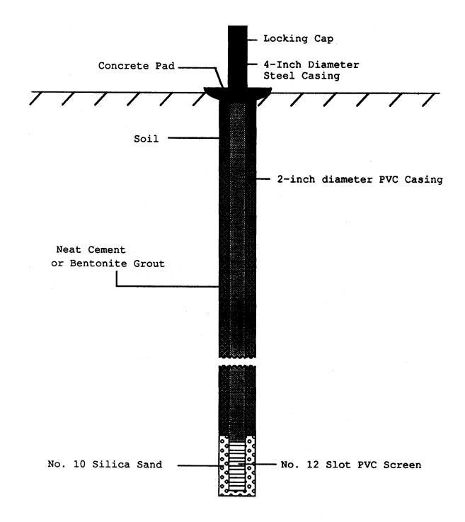
Figure 2. Construction design used for monitoring wells installed at the Devils Lake landfill.
