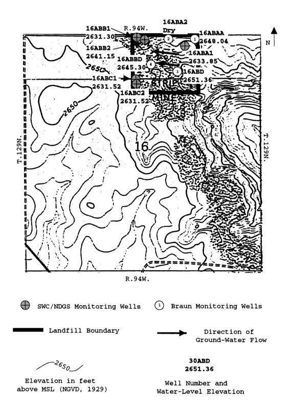
Figure 4. Location of monitoring wells and the direction of ground-water flow.
