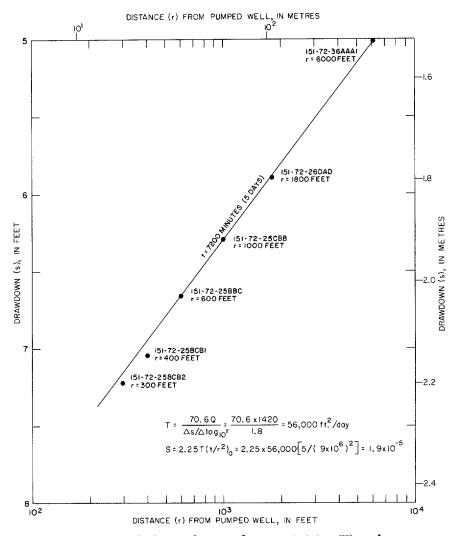
FIGURE 14.— Straight-line solution of transmissivity (T) and storage coefficient (S), New Rockford aquifer test (1969).
