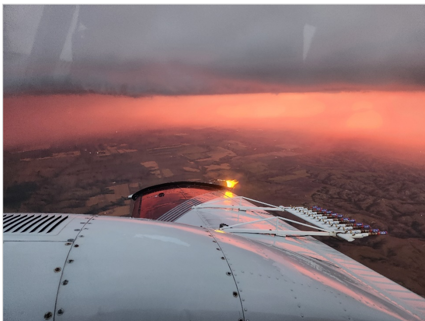
Fig. 38. N121WA with a burner lit seeds a storm over McKenzie County on a late summer evening (July 30 th , 2023). Photo by Laura Standen.
